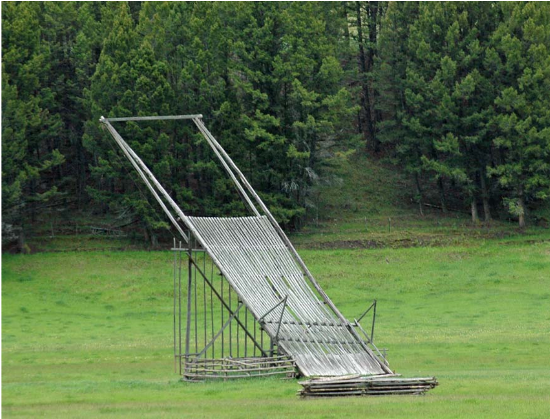
Figure 17. Beaverslide made of timber near Avon, Montana. June 2009. Photo: Linnea C. Sando.
