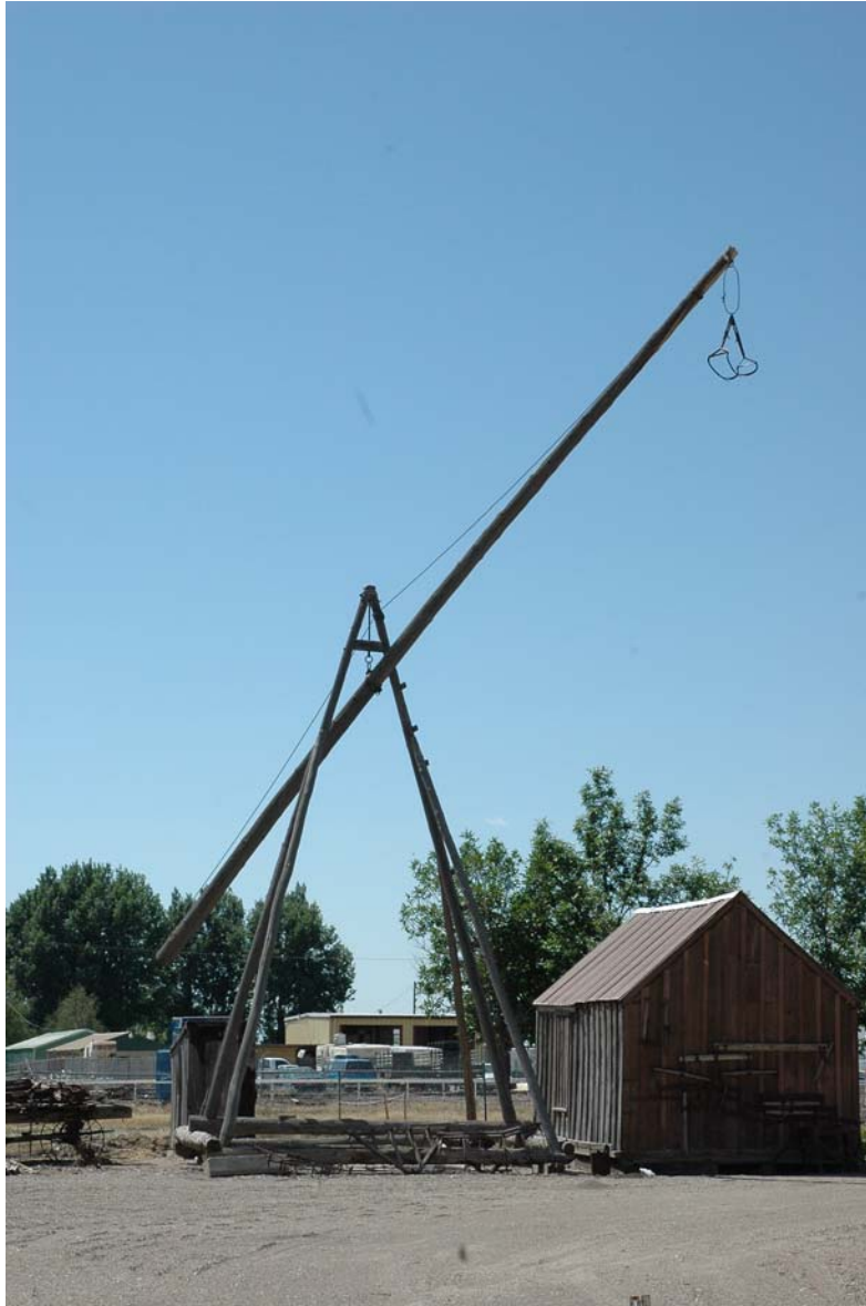
Figure 3. Hay derrick outside of museum near Rupert, Idaho. June 2009. Photo: Linnea C. Sando.
