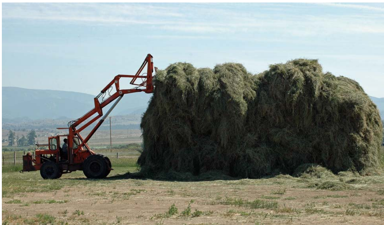
Figure 62. Special tractor with a front loader extension to stack hay loosely. July 2009, Helena, Montana. Photo: Linnea C. Sando.
