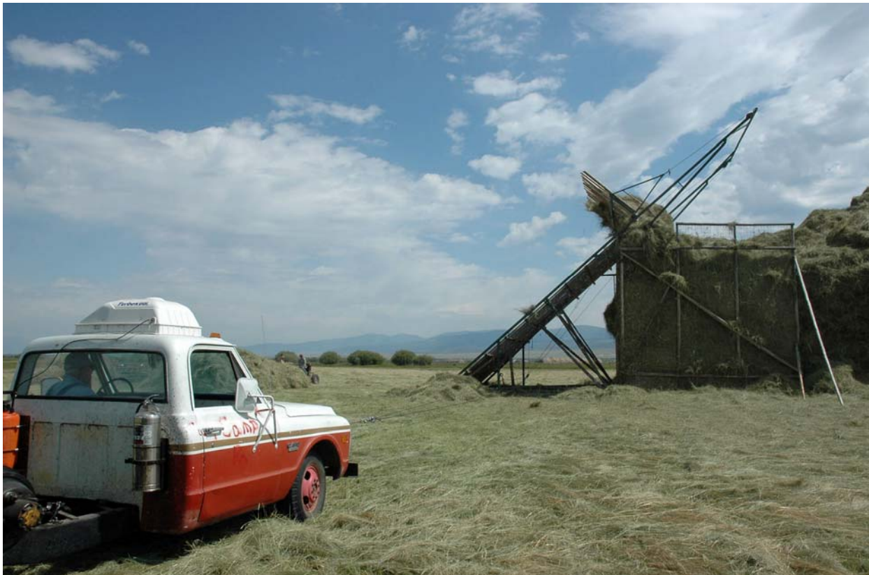
Figure 19. Truck providing power to lift the Beaverslide's toothed basket. The truck is connected to the basket with cables. It provides power to pull the cables and raise the loaded basket to the top. July 2009, Jackson, Montana. Photo: Linnea C. Sando.
