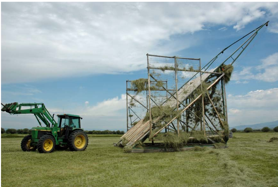
Figure 22. Skids on bottom of Beaverslide allow for an easier transport to the next hay field. July 2009, Jackson, Montana. Photo: Linnea C. Sando.
