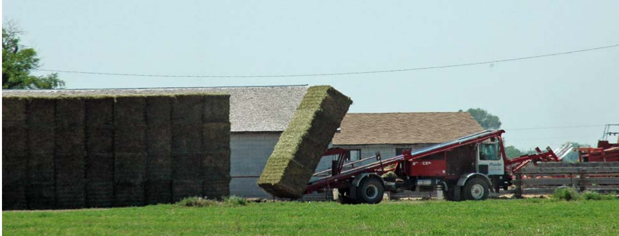
Figure 54. Truck stacking multiple bales at once. June 2009, southern Idaho. Photo: Linnea C. Sando.
