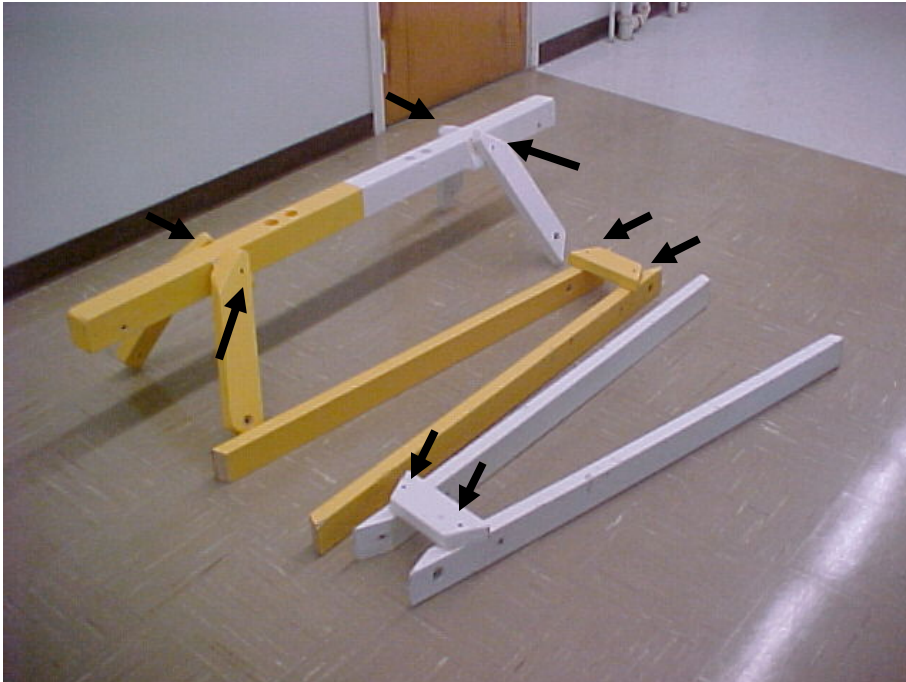
Figure 5 Structural Components: Parts Pivot on Permanent Screws (Arrows)
