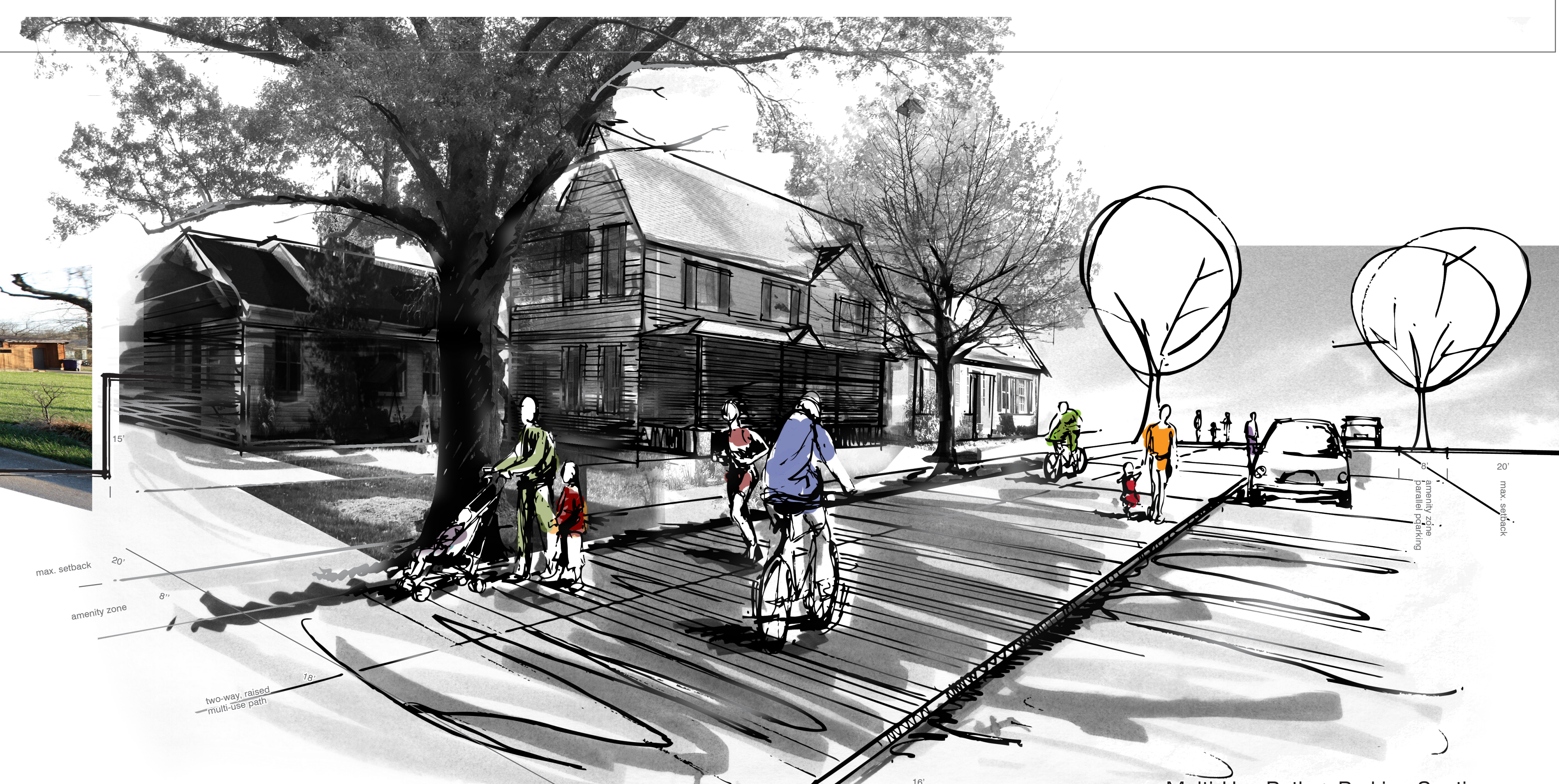
Multi-Use Path + Parking Section emphasizes physical activity in residential neighborhoods by 18-ft wide two-way multi-use path and narrow 16-ft wide two-way vehicle travel lane
