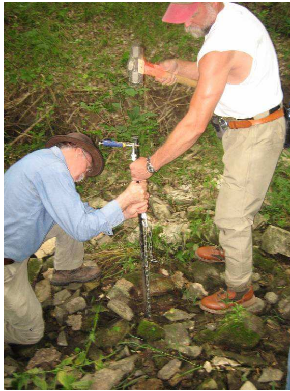
Figure 2-16. Installing a scour chain at riffle on Wind Creek, upland reach.
