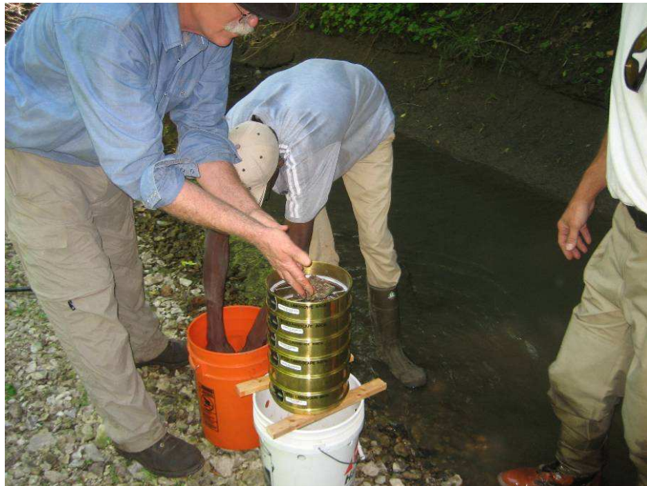
Figure 2-15. Sieve analysis of a bar core sample at Silver Creek, Keats.
