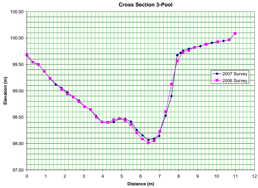
Figure A-20. Repeat survey of cross section transect 3 at Farnum Creek.
