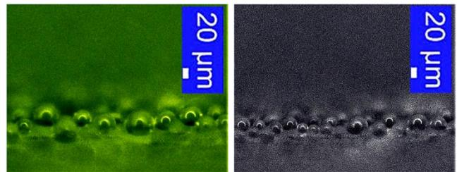
**Figure 7.** Droplet growth images for Teflon® coated nanopillar surface. Spherical cap shaped condensed droplets with average contact angle greater than  $90^\circ$  have been observed (side-view).
