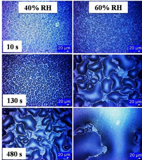
**Figure 4.** Time-lapsed droplet growth on plain Ti pillared glass surface at 40% RH and 60% RH respectively
