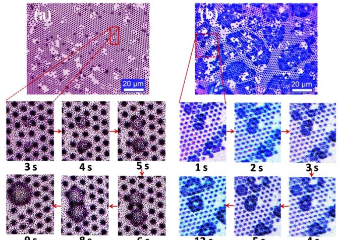
**Figure 6.** The wetting state was evaluated based on the images recorded for the droplet growth in a unit cell (a) hydrophobic surface, 30 % RH (b) plain Ti pillared surface, 40% RH.
