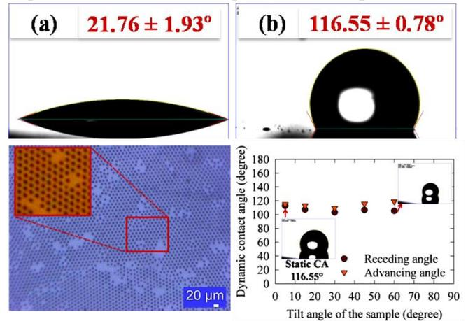
Figure 2. Static and dynamic contact angle measurement on (a) plain Ti pillared (b) Teflon® coated Ti pillared glass surfaces
