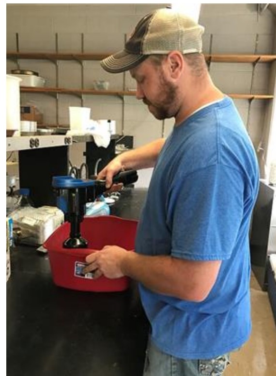
Figure 3.2 Scanning sample with NIR device
