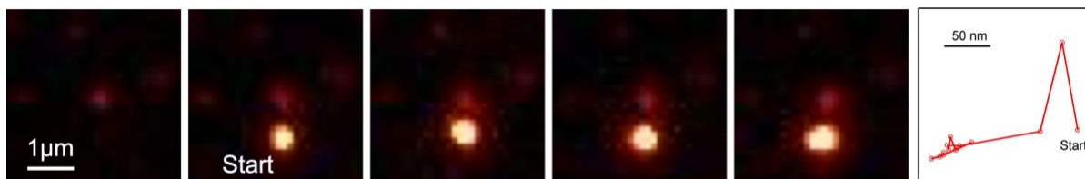
Figure 4.6 Consecutive video frames showing the initial adsorption and residual motion (left to right) of a single plasmid DNA molecule at +1.4 V in the near-monolayer region (8.8 mm) of the gradient, under pH ~ 8 buffer. A plot of the DNA position across several frames is shown at the far right. The DNA molecule fully adsorbs to the surface after the fourth frame.
