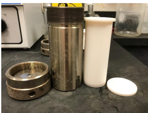
Figure 1-2: Parr Teflon-lined stainless-steel bomb with a capacity of 45 mL: acid digestion vessel (left), PTFE cup (right)
