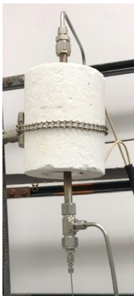
Figure 5-2: The stainless-steel 316 tube reactor and furnace setup in the hood
