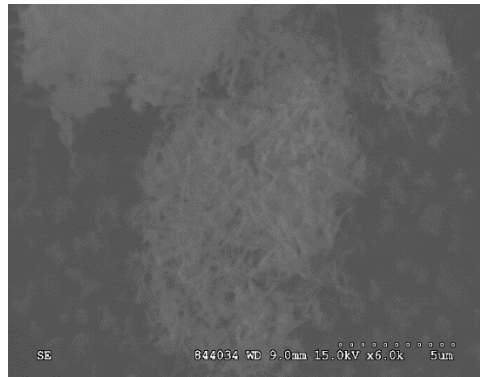
Figure 3-22: SEM of short calcined VPI-8 synthesis synthesis at 200 °C for 6 hours, reaction composition: 0.2 LiOH : 0.1 Zn(CH 3 COO) 2 ·2H 2 O : 0.4 TEAOH : SiO 2 : 30 H 2 O (exp.1)
