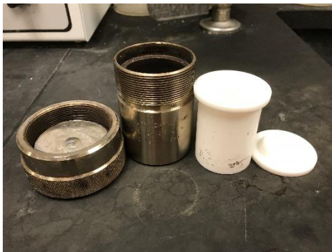
Figure 1-1: Parr Teflon-lined stainless-steel bomb with a capacity of 23 mL: acid digestion vessel (left), PTFE cup (right)
