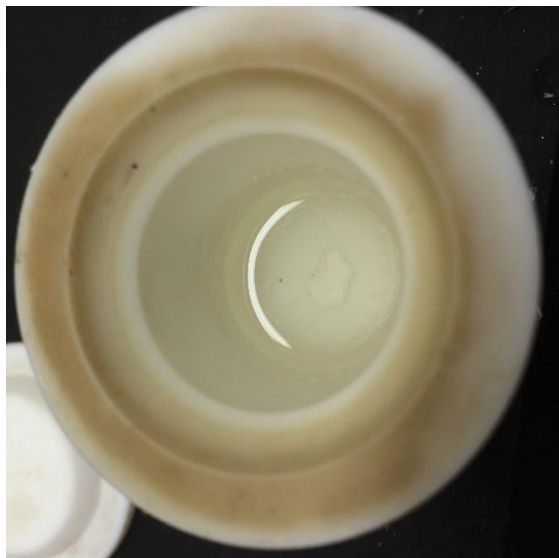
Figure 3-20: Product picture of with-seed synthesis, a hard disk format lay at the bottom of the reactor (exp. 18)
