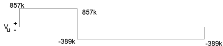
Figure 5.23 – STM Design Example 2 - Shear Diagram
