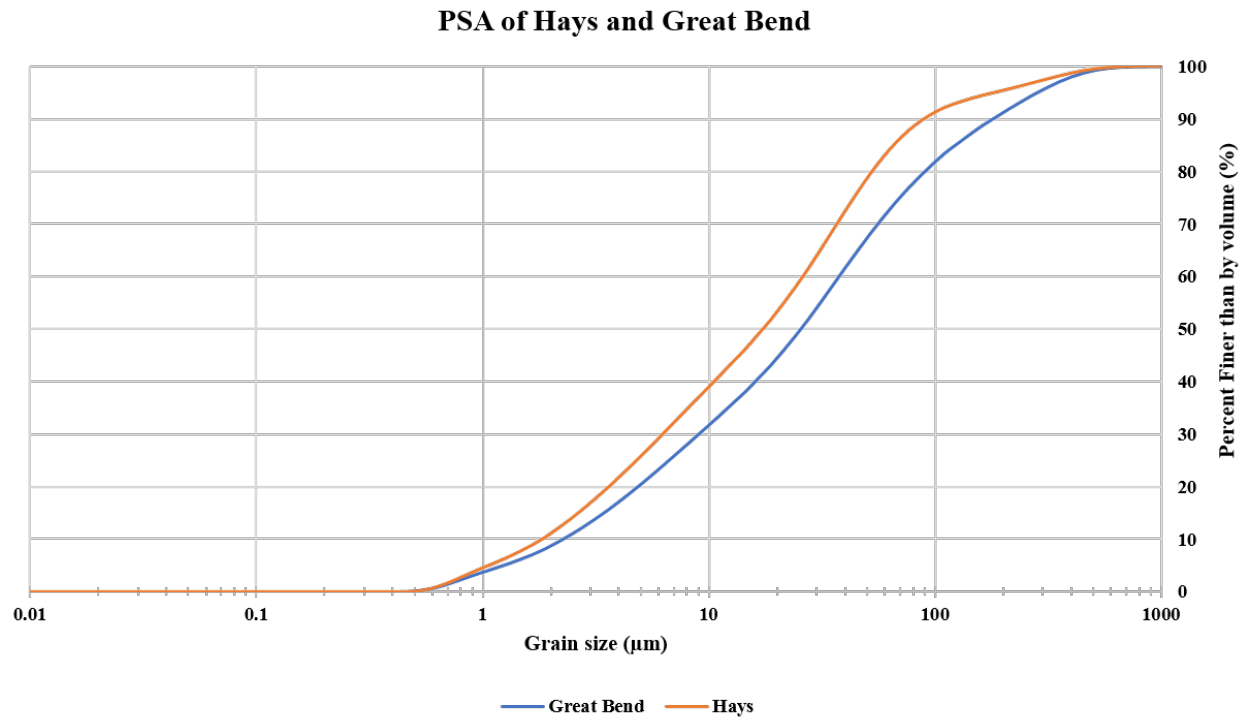
Figure 4-4: Cumulative particle grain size of Hays and Great Bend
