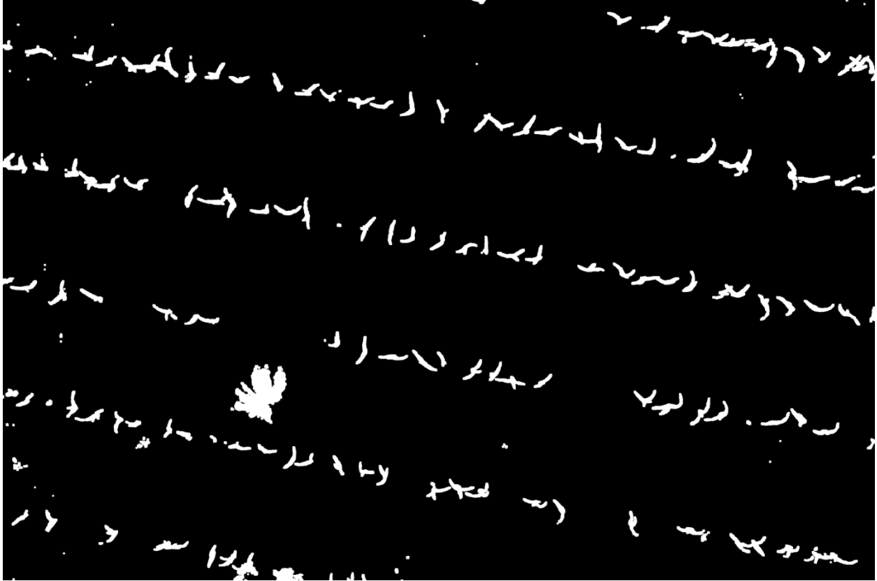
Figure 3. Image obtained after applying ExG segmentation and Otsu's thresholding
