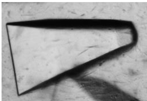
Figure 2.2. A typical tomahawk shape of lactose crystal. Stable and Unstable \alpha -Lactose Anhydrous
