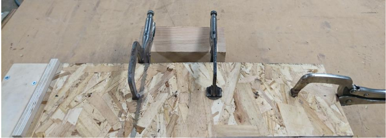
Figure 4-4 Wood Panel Clamped on the Top of the CFS flange
