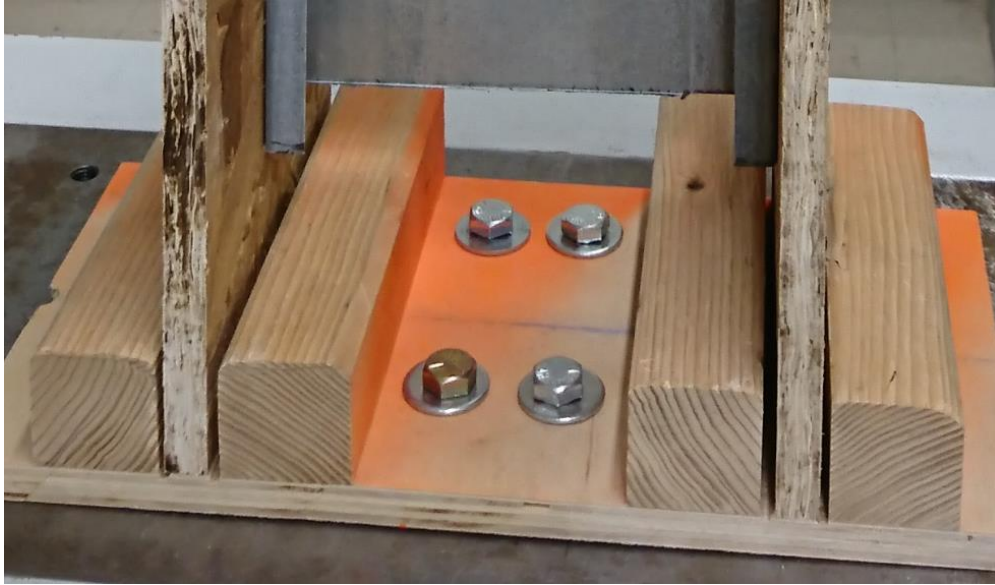
Figure 3-3 Base Plate Bolted to the Testing Machine
