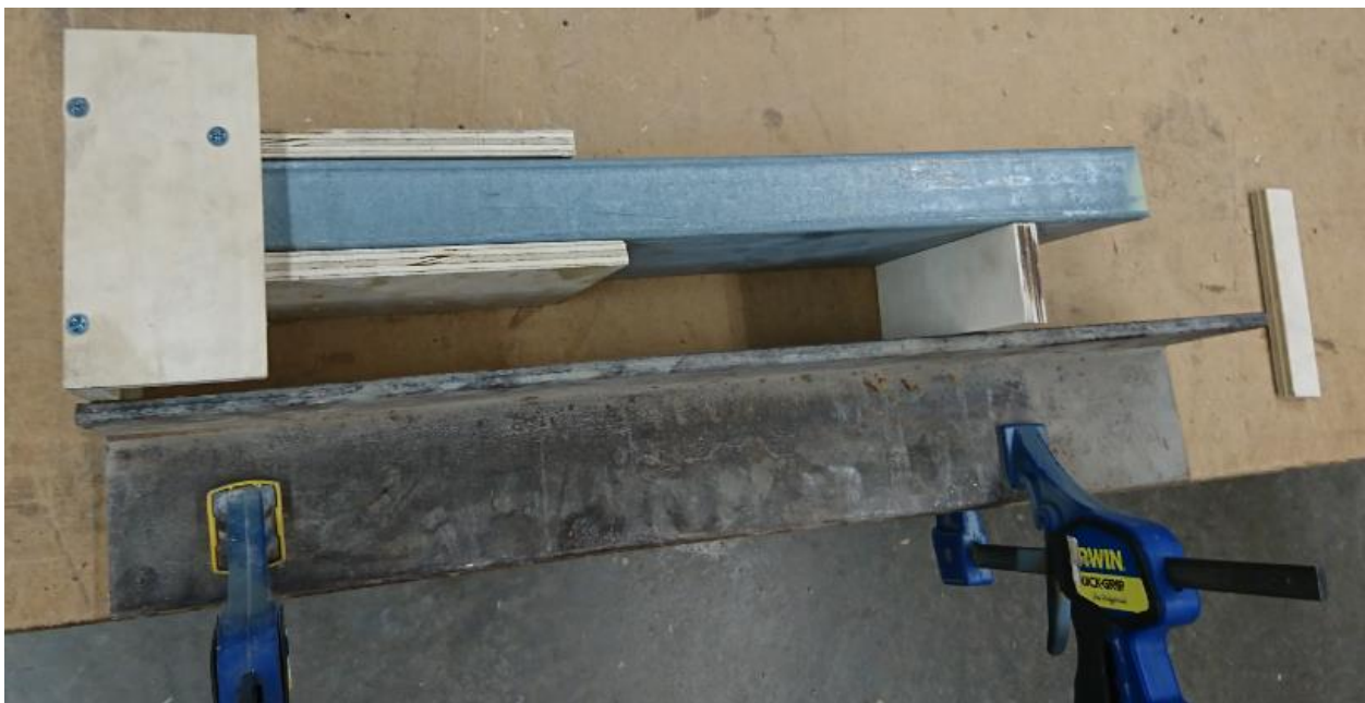
Figure 4-3 CFS Regulated by Wood Jig and a Piece of Wood
