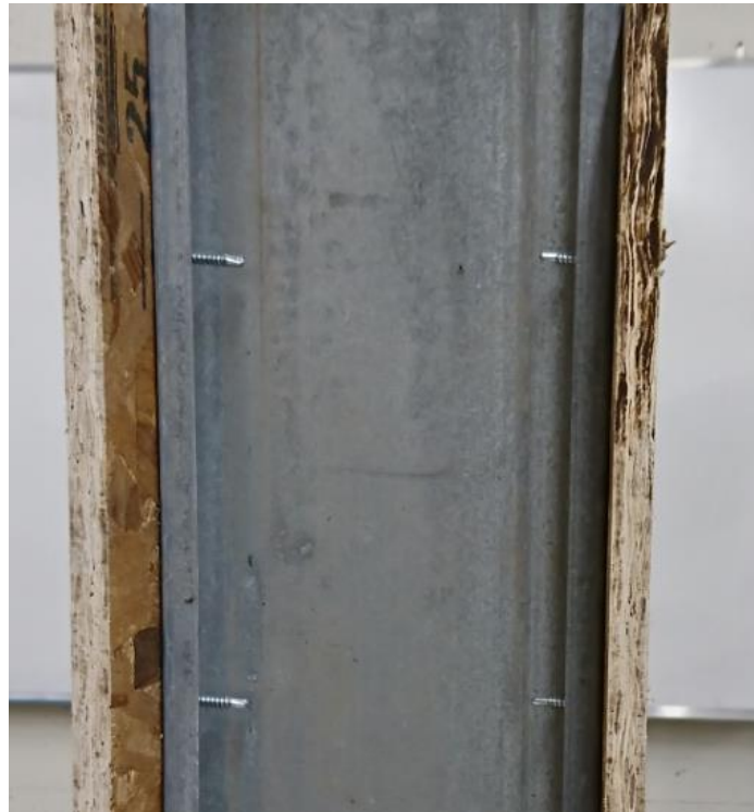
Figure 4-6 Specimen with Screws installed Non-Perpendicular to the Sheathing
