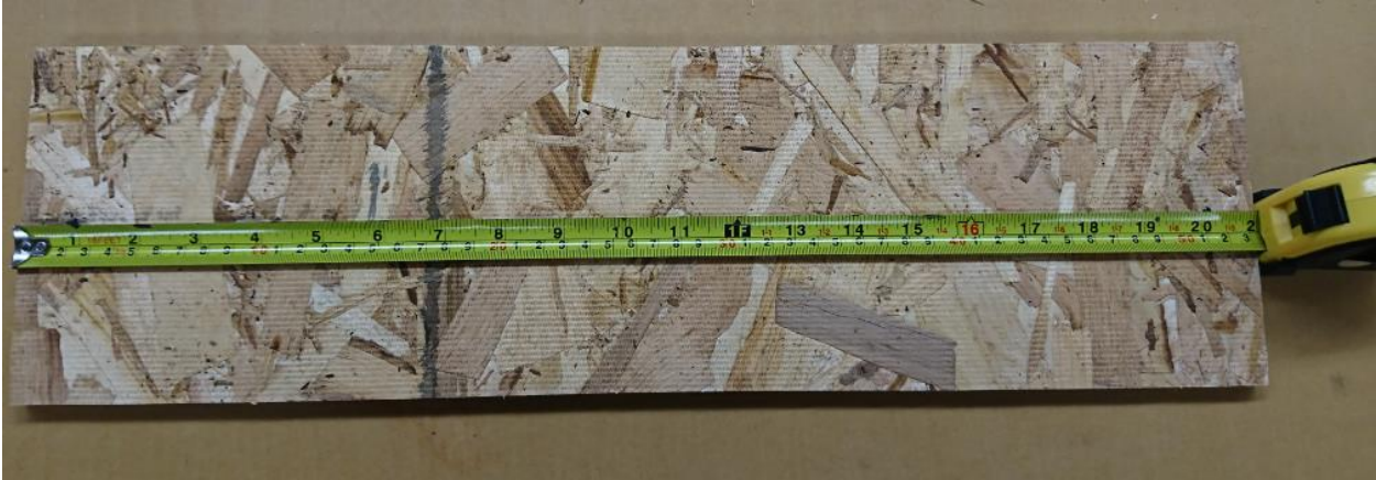
Figure 4-2 Marking Screw Locations on Timber Panel
