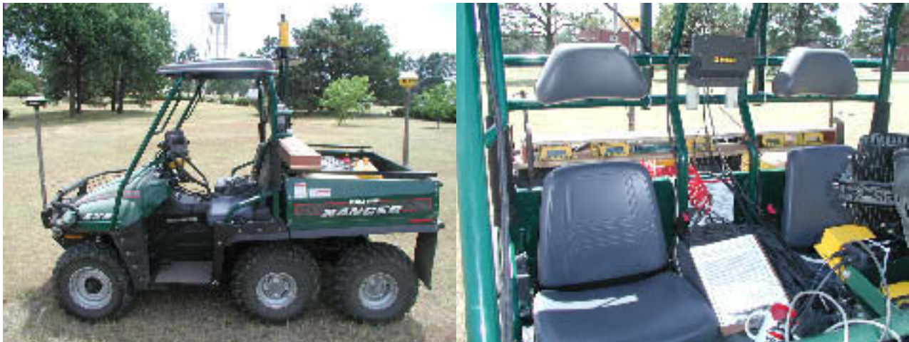
Figure 2-2 (left). Rover vehicle used for the dynamic test showing primary (front) and secondary (rear) antennas.
