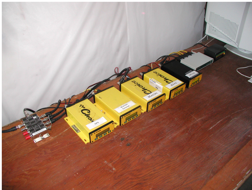
Figure 1-3. Antenna splitter, GPS receivers, and RS-232 multiplexer arrayed for the static test.
