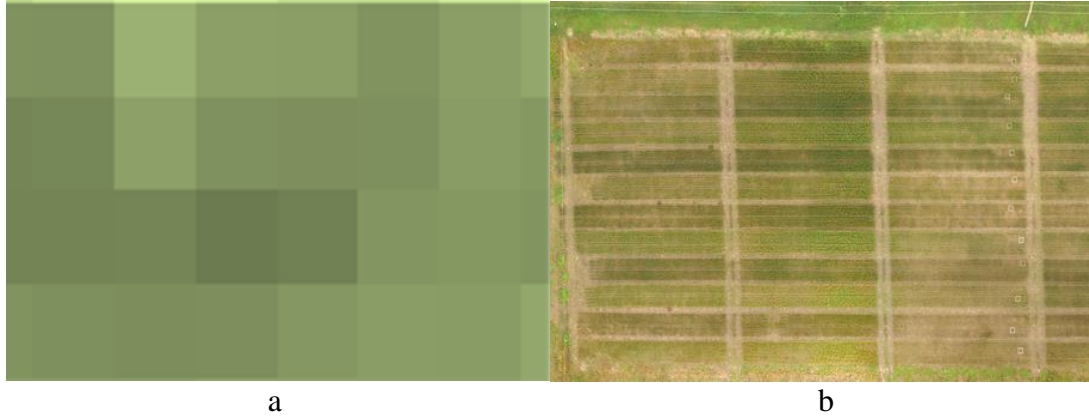
Figure 1.5 Examples of a coarse resolution and a fine resolution image taken at the same field. a. 2 cm resolution RGB image taken at 60 m above ground level (AGL); b. 10 m resolution RGB image taken by Sentinel-2.
