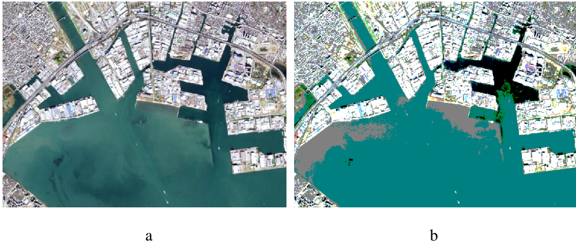
Figure 1.6 Different radiometric resolution. a. 8-bit Sentinel-2 image; b. 2-bit Sentinel-2 image.
