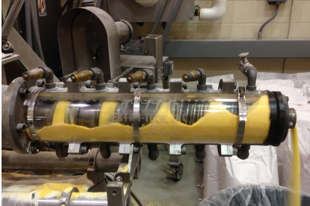
Figure A-5 Corn Meal at Steady State (13.13% Moisture)
