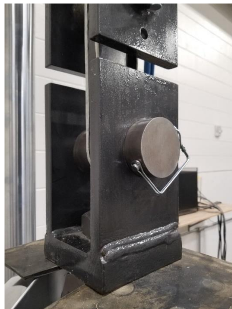
Figure 15. Steel pin used for tensile test
