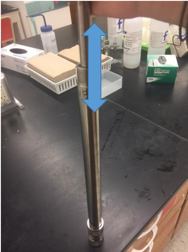
Figure A-4 Tamping wool, sample, and glass beads or matrix in vessel with rod
