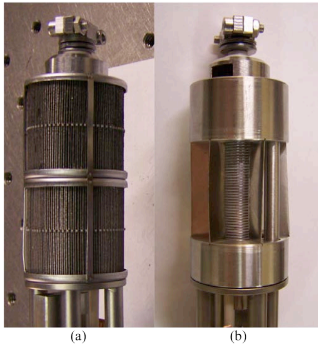
Figure 4.12 The original GP50 (a) with 32 grams of ST-707 shown next to the redesigned getter (b). The redesign uses 6 pieces of ST-707 for a total mass of approximately 1 gram.
