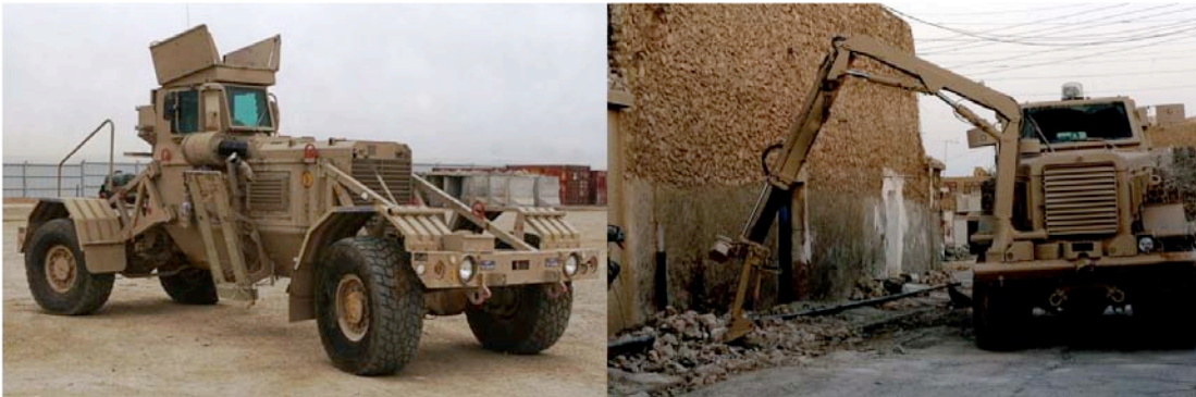
Figure 1.2 A Husky Mine Detection Vehicle (left) and a Buffalo MPV (right).
