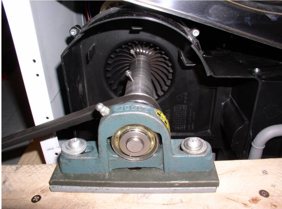
Figure 4.2 Drum Motor Coupling Shaft and Pulley System
