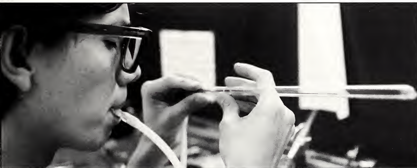
With an eye for detail, Alvaro Herrera, graduate student in biochemistry, breathes air through a blow hose into the pieces of glass he is attempting to straight-seal together. "What interested me about the class was being able to learn how to do things with your hands," Herrera said. Photo by Lindsey Bauman
