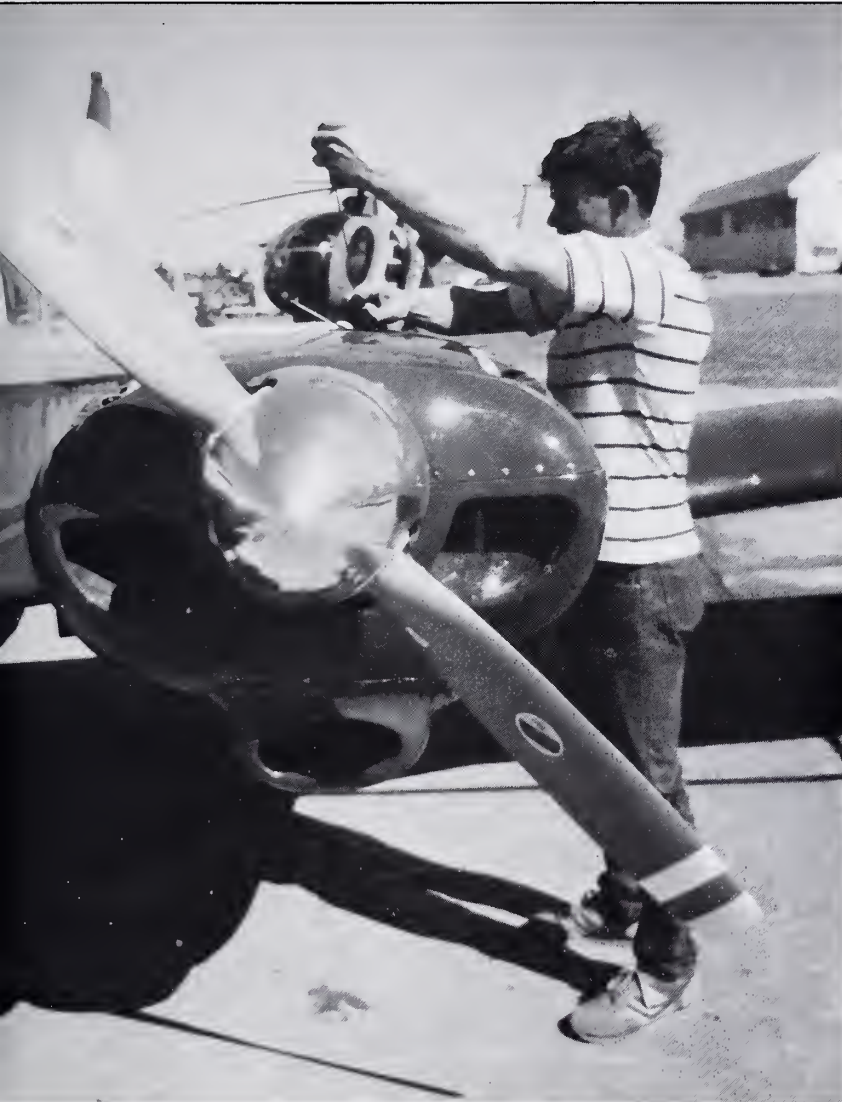
ABOVE: Mike Hamden, AM, checks the oil in one of the engines on a twin engine aircraft as part of the aircraft maintainance program at Kansas Tech.
