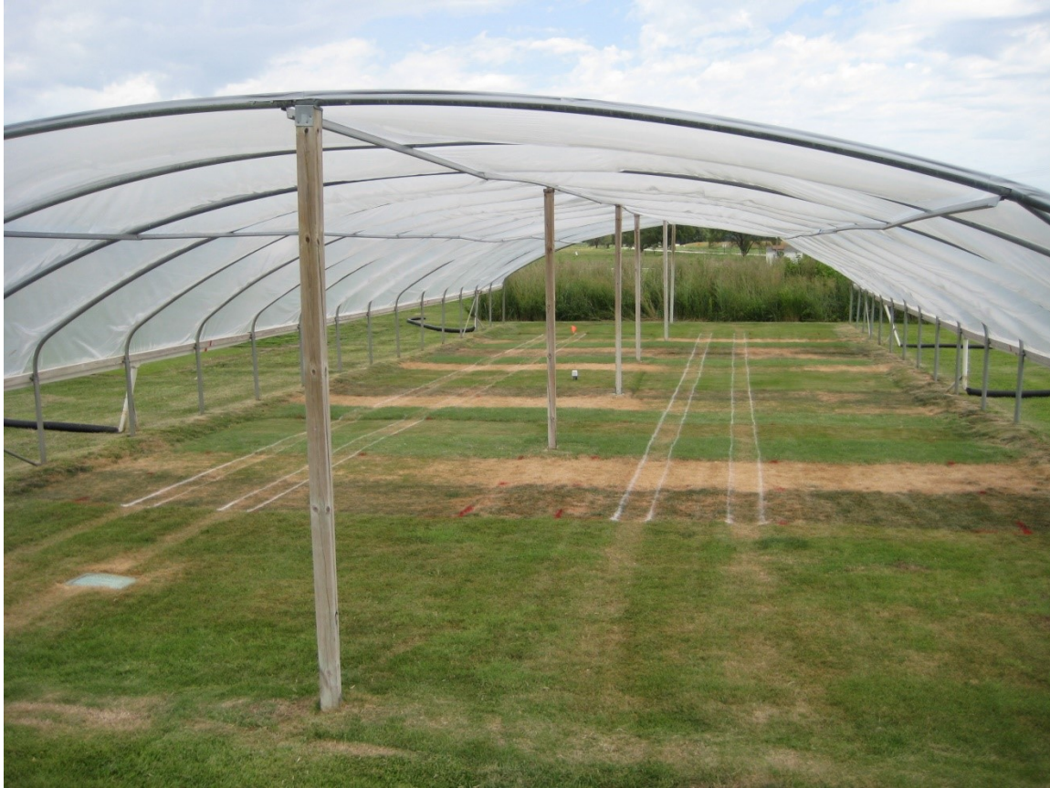
Figure B.2. Field plots at Rocky Ford Turfgrass Research Center, Manhattan KS on 6 Aug. 2016 (41 days of simulated drought with no irrigation and a total of 96 golf cart traffic passes applied inside the white lines).
