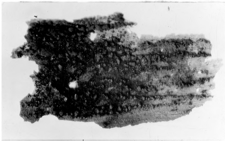
Figure 1. A coke-like chip showing the condition in the carburizing retort when the gases are dry. X 2.
