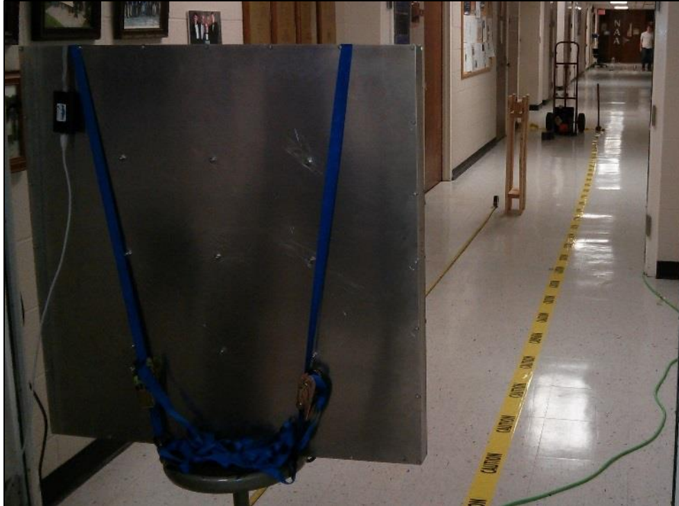
Fig. 6.4.5. The Panel Array Mk II was tested for neutron sensitivity in a concrete hallway at distances of 1 m, 2 m, 5 m, and 10 m. A 54 ng ^{252}\text{Cf} source with a neutron activity of approximately 125,000 \text{ n s}^{-1} at 1 m above the floor was used for the sensitivity measurements.
