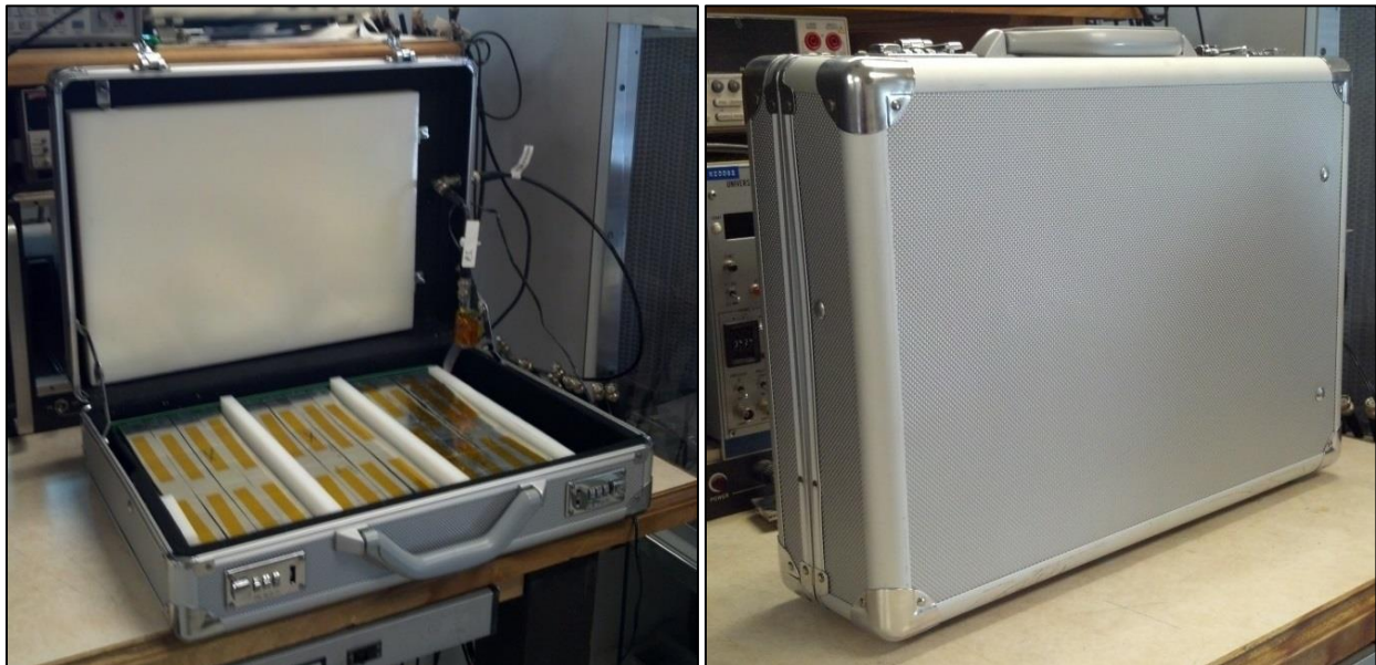
Fig. 5.1.12. Depicted is the Briefcase Neutron Detector system. The system uses twelve or twenty-four strings of seven Dominoes tiled laterally to form a large-area, man-portable thermal neutron detector system. The Dominoes are sandwiched between two 1-in. thick sheets of HDPE moderator.
