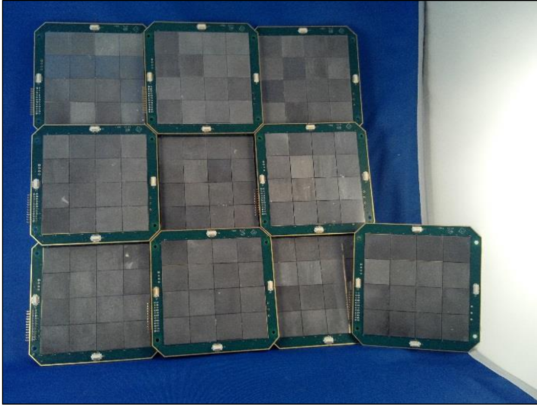
Fig. 5.1.3. The individual 4x4 elements were tiled into a 3 x 3 array and made to function as a single, large area detector with a total active neutron detection area of 144 cm 2 .
