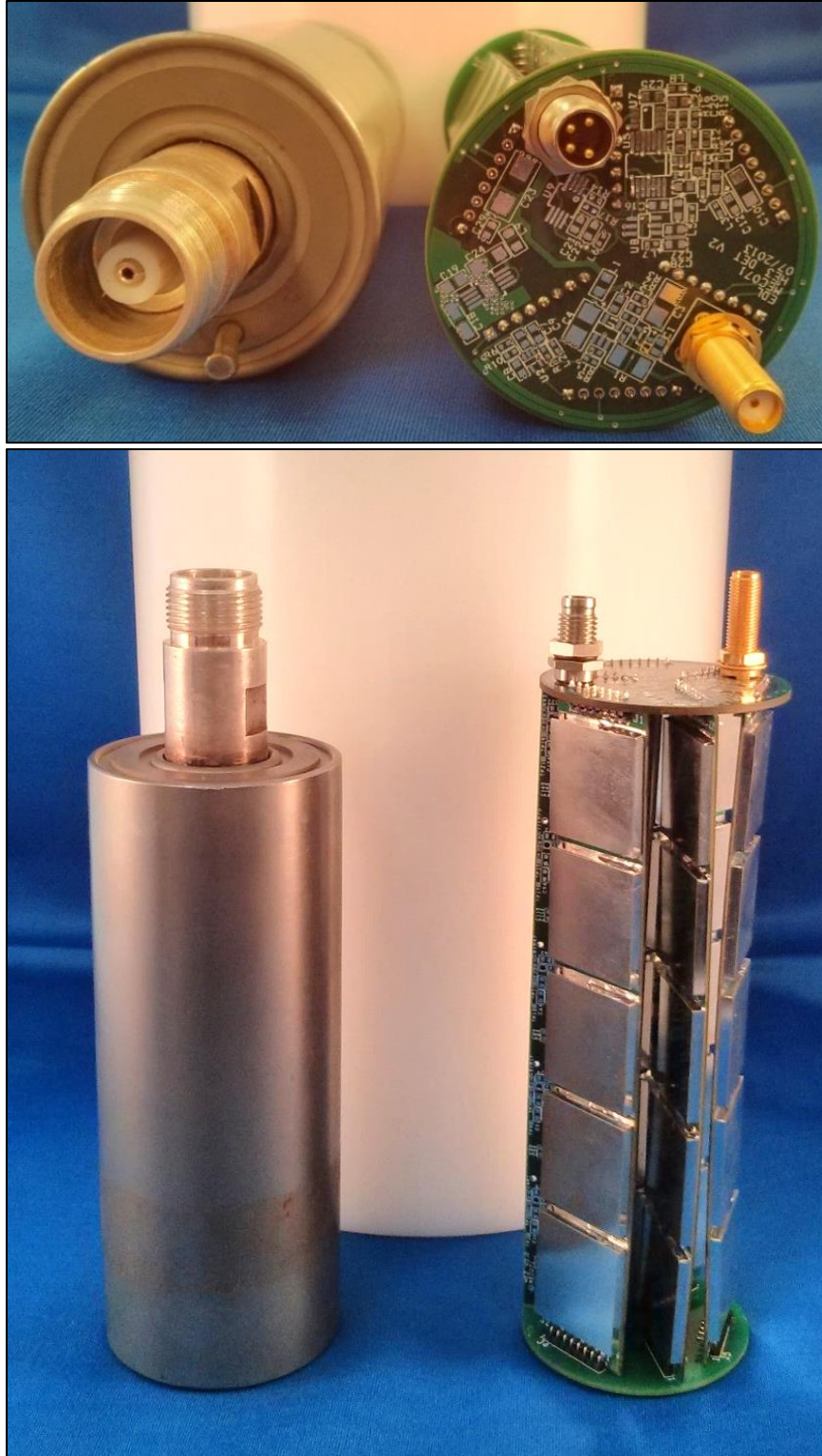
Fig. 5.2.2. The second generation Helium-3 Replacement (HeRep Mk II) detector was developed in 2013 and refined in 2015. The HeRep Mk II was populated with thirty 4-cm 2 active area MSNDs, each with an intrinsic thermal neutron detection efficiency of 20% (and later 30%), arranged in six strips of five sensors each. The detector was intended to directly replace a 2-in. diameter, 6-in. long 3 He pressurized to 4 atm.
