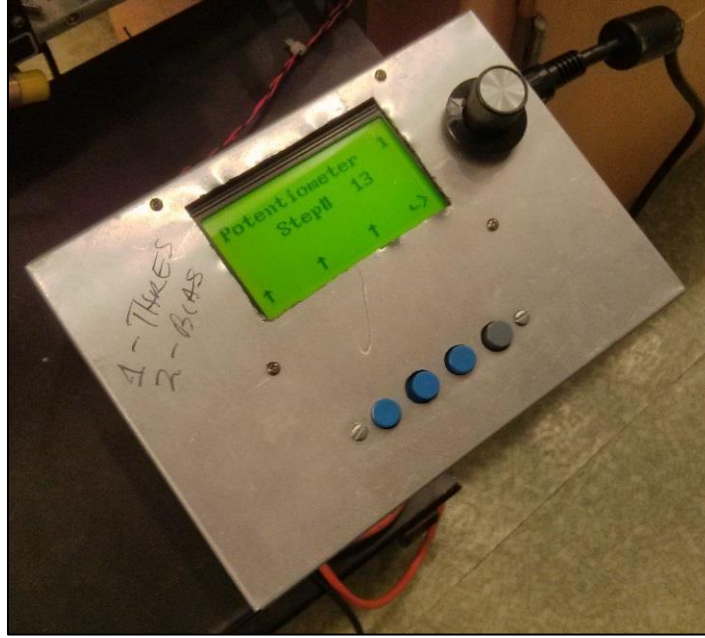
Fig. 5.2.4. The HeRep control box allows for a user to program the applied bias and the threshold settings for the entire HeRep device. Applied bias can be globally adjusted from 0 V to 5 V in 0.2 V increments, and the discriminator threshold values from 0 V to 2 V in 4 mV increments. The programming box can be removed from the system following the settings adjustment.
