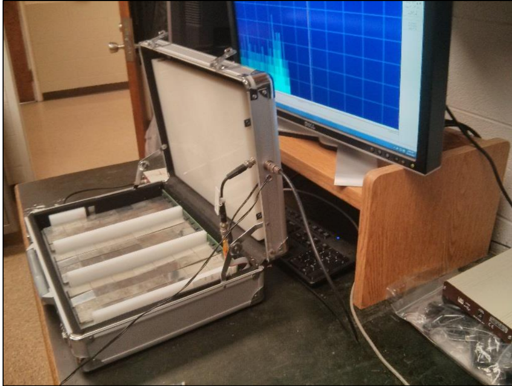
Fig. 6.4.2. Shown is the Briefcase Neutron Detector during a 24-hour-long background measurement. The test was intended to measure the long-term background stability of the detection system by conducting a measurement of the supposedly stable neutron background.
