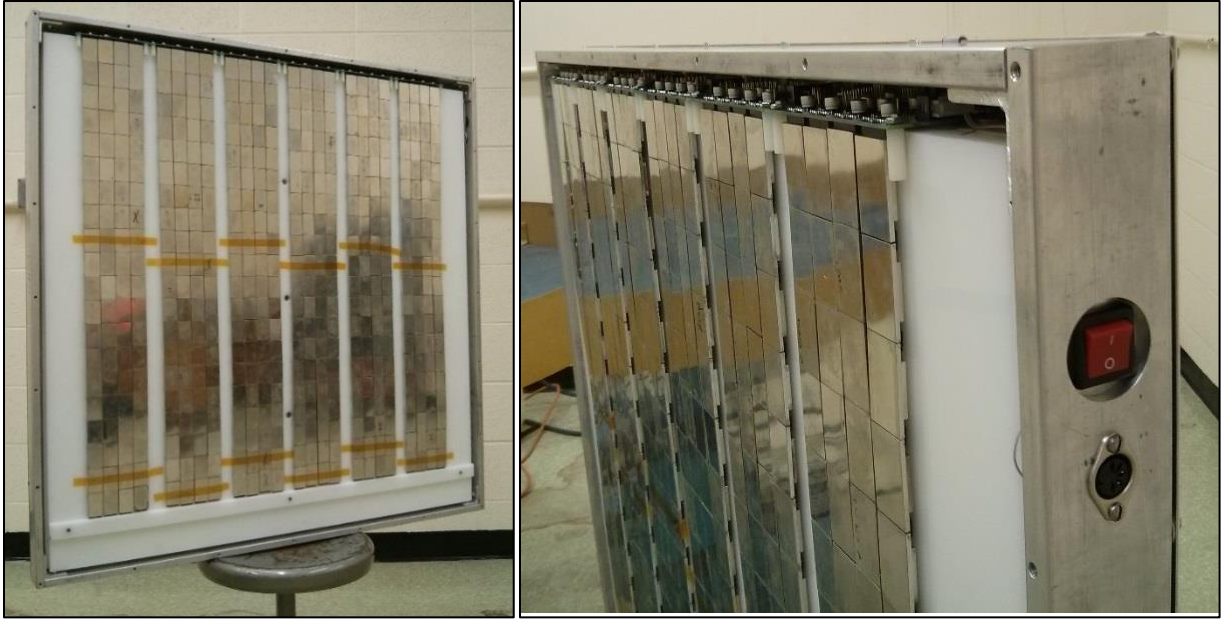
Fig. 5.1.14. Shown is the Panel Array Mk II neutron detector system that utilized twenty-four strings of twenty Dominoes, sandwiched between two 1-in. thick sheets of HDPE moderator to form a 1 m x 1 m detector array.
