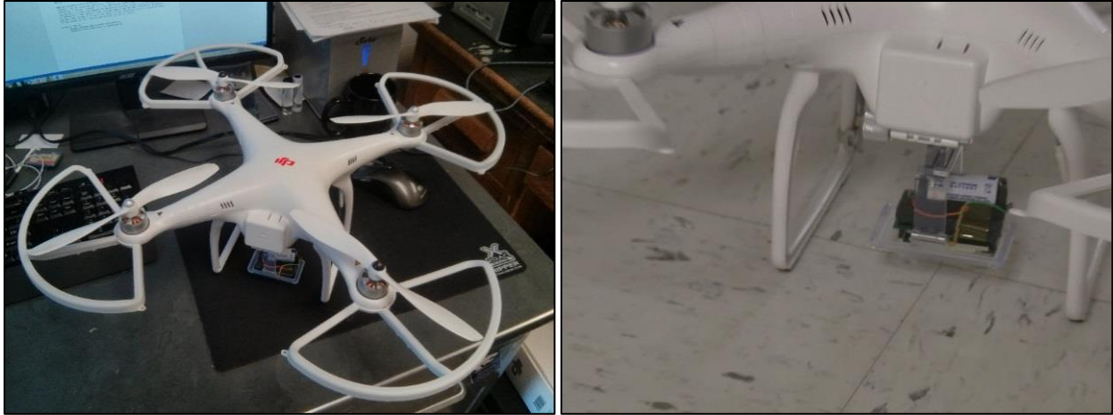
Fig. 5.1.10. Shown is a Domino coupled with a wireless Bluetooth electronics package paired with a DJI Phantom drone for remote source investigation.
