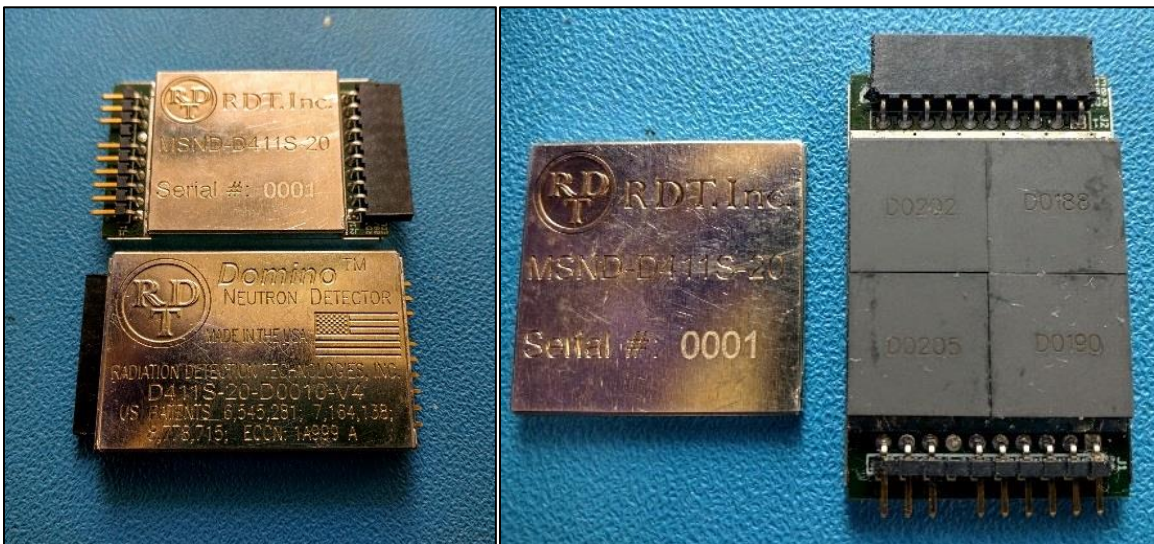
Fig. 5.1.7. Shown (left) is the Domino TM modular neutron detector with its front-facing RF shield removed, and (right) displaying the four underlying 1-cm 2 active area MSNDs.
