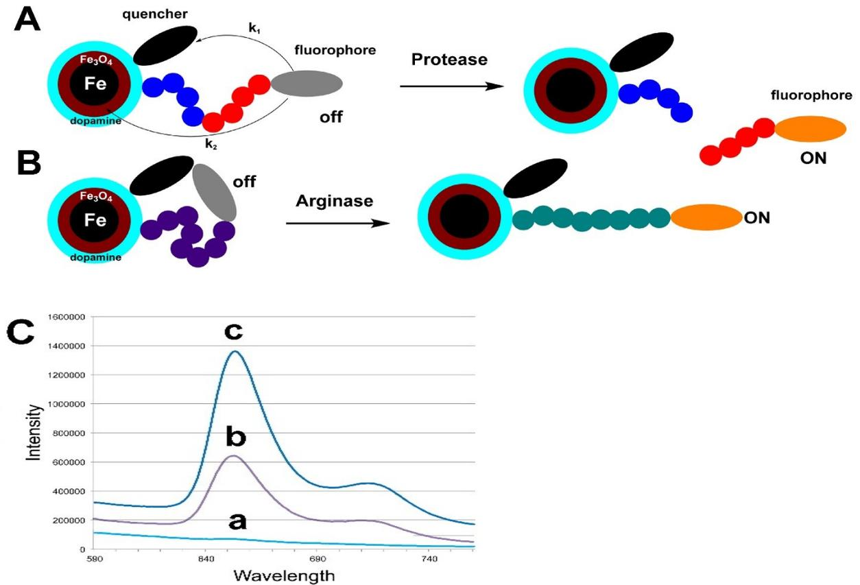
**Figure 5: A: Function principle of nanobiosensors for protease detection: the consensus sequence is cut by the protease; B: Function principle of nanobiosensors for posttranslational modification: the chemical identity of amino acids in the linker is changed via enzymatic reaction; C: Typical emission spectra occurring from the nanosensor for MMP-3 after 1h of incubation at 37°C ( $\lambda_{exc} = 421\text{nm}$ ). a: buffer; b: nanosensor; c: nanobiosensor after incubation with MMP-3**
