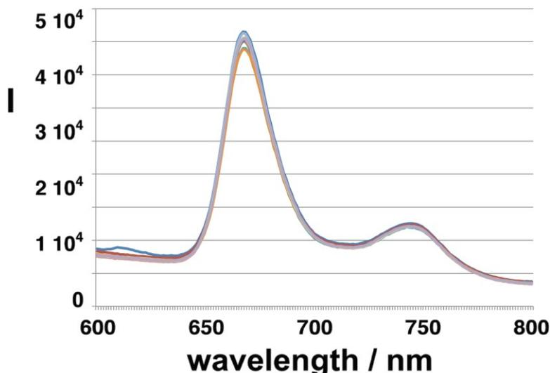
**Figure 51:** 10 independent repetitions of measuring the activity of the Fe/Fe<sub>3</sub>O<sub>4</sub>-nanoplatform for detecting MMP-13 under standard conditions at 25 °C after addition of 1.0 x 10<sup>-13</sup> mol L<sup>-1</sup> of MMP13. The relative error was determined to be 2 percent. I: fluorescence intensity
