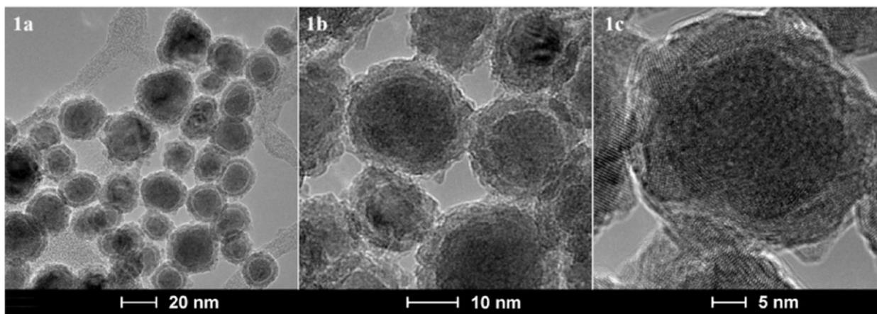
Figure 49: “TEM (1a,1b) and HRTEM (1c) images of Fe/Fe<sub>3</sub>O<sub>4</sub>-core/shell nanoparticles that are forming the inorganic core of the nanoplatforms for protease detection, HRTEM images revealed that the Fe(0) centers are mostly crystalline (BCC).”<sup>122</sup> (Taken with permission of the Royal Society of Chemistry<sup>122</sup>)
