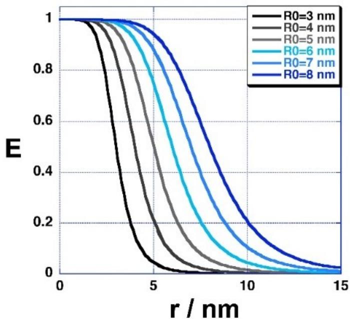
**Figure 4: Energy transfer efficiency  $E$  as a function of the distance between donor and acceptor (nm), and the Förster radius  $R_0$**
