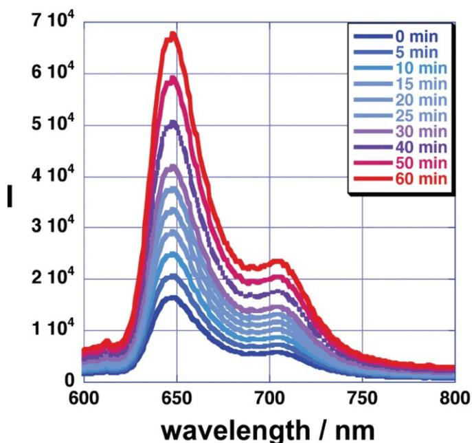
Figure 50: “Light-Switch Effect” of the Fe/Fe<sub>3</sub>O<sub>4</sub>-nanoplatform for detecting MMP-13: fluorescence increase as a function of reaction time under standard conditions at 25 °C after addition of  $1.0 \times 10^{-12}$  mol L<sup>-1</sup> of MMP-13; I: fluorescence intensity (Taken with permission from Royal Society of Chemistry<sup>122</sup>)
