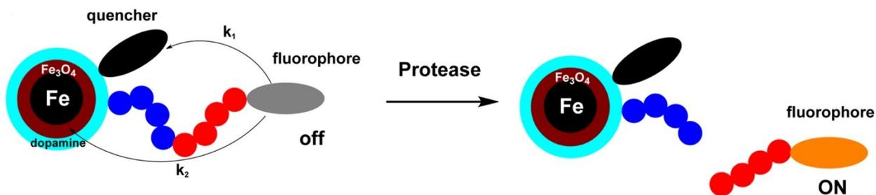
**Figure 33: Mechanistic scheme of the “light switch effect” upon proteolytic cleavage. The fluorophore is switched on due to the increase in distance between the Fe/Fe<sub>3</sub>O<sub>4</sub> core/shell nanoparticle, leading to decreased Förster Resonance Energy Transfer (FRET),  $k_1$ , and dipole-surface energy transfer (SET),  $k_2$ .**
