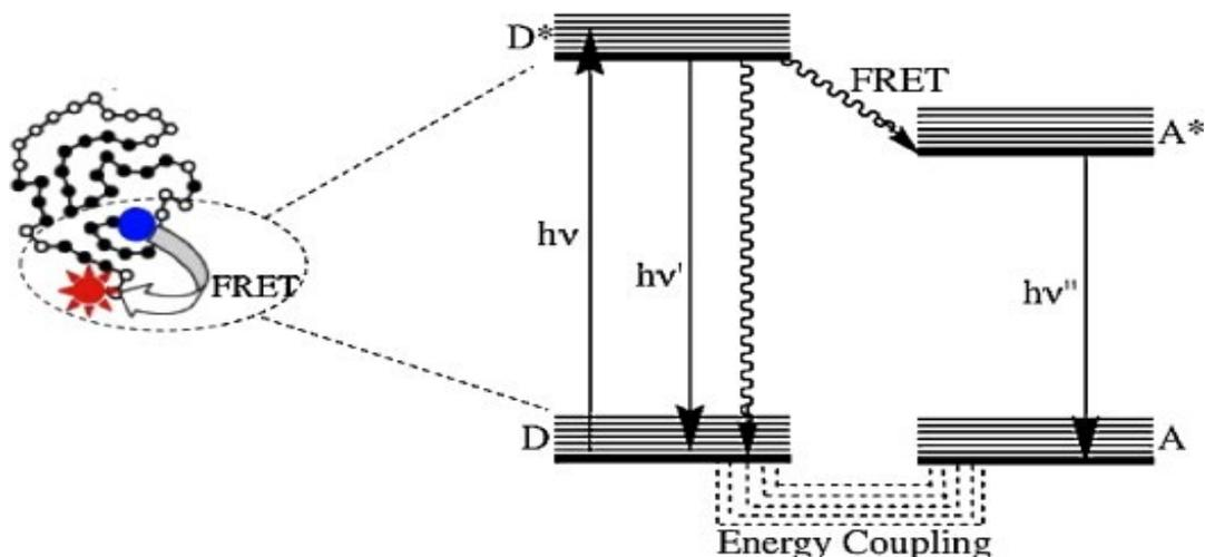
**Figure 2: Schematic representation of FRET demonstrating the energy transfer from excited donor (D\*) to acceptor (A) via nonradiative process. Note that external conversion of the acceptor is not shown (Taken with permission of Reference <sup>12</sup>)**
