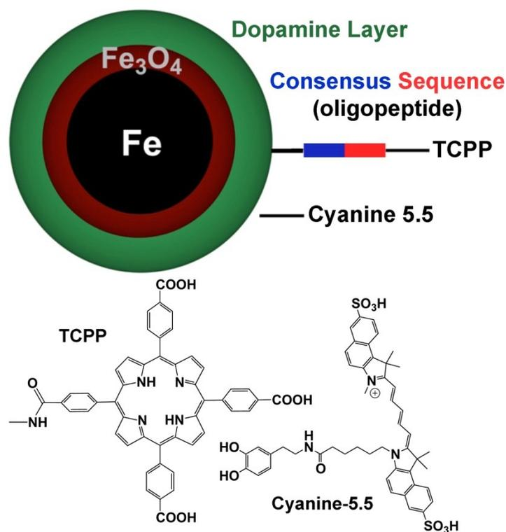
**Figure 34: Nanobiosensor for in-vitro protease detection.** For each protease, a highly selective consensus sequence is employed as a tether between nanoparticle and TCPP (tetrakis-4-carboxyphenyl-porphyrin). Cyanine 5.5 is linked permanently to the Fe/Fe<sub>3</sub>O<sub>4</sub> nanoparticles. Cited from reference <sup>122</sup> with permission from the Beilstein Journal of Nanotechnology.
