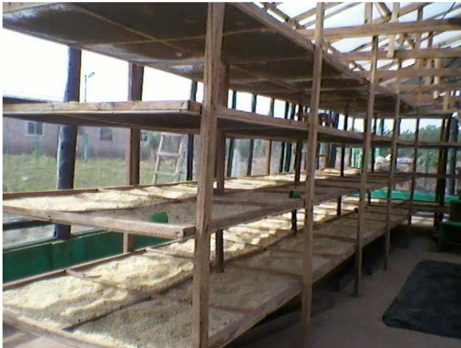
Figure 2: Shelves stacked with maize harvest in the biomass hybrid solar dryer in Ejura, Ghana.
