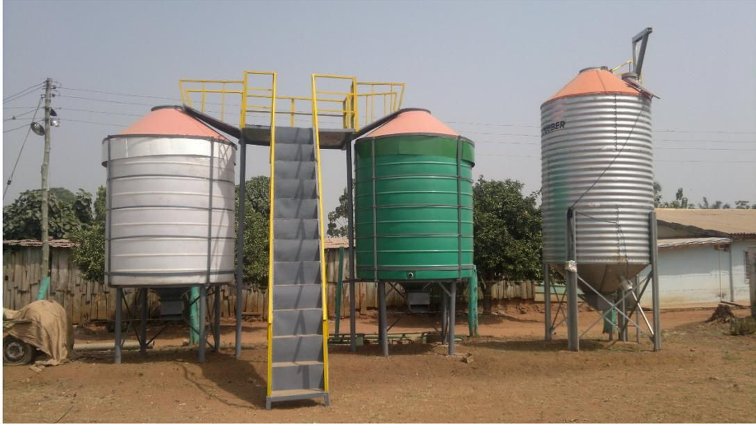
Figure 3: Plastic water tanks modified into silo for long term storage of maize in Ejura, Ghana (metal silos on the right was donated from a Brazilian company and additionally tested).
