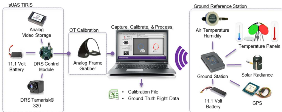
Figure 4.9. TIRIS component system diagram for camera calibration and ground reference data
