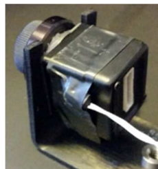
Figure 2.6. Thermistor mounted to camera housing temperature for subsequent testing
