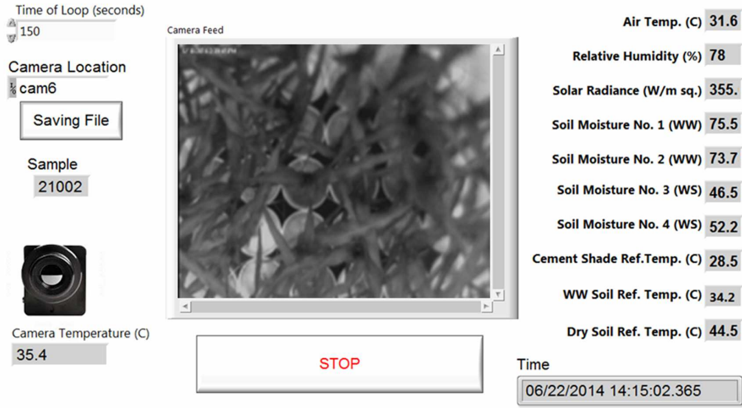
Figure 3.5 Greenhouse TIRIS VI front panel for controlling loop time and camera control while monitoring and saving soil moisture of irrigation regimes, air temperature, relative humidity, solar radiance, reference panels, camera temperature, sample number, and time stamp.
