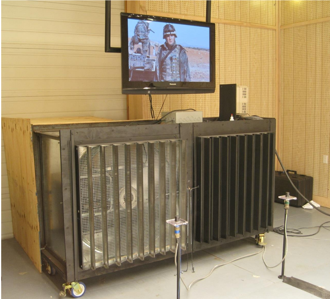
Figure 8.10 Fans, air temperature sensors, humidity sensors, and TV
