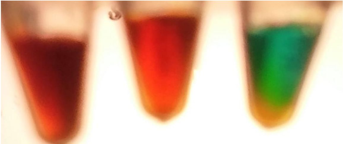
Figure 9. Hemoglobin powder assay optimization in tubes. From left to right: 16 g/dL, 12 g/dL, 8 g/dL.
