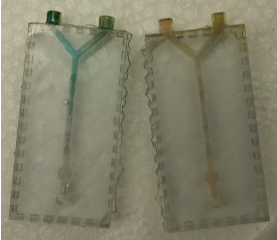
Figure 11. Complete mixing hemoglobin powder solution and assay in Chip B. (8 g/dL and 16 g/dL)
