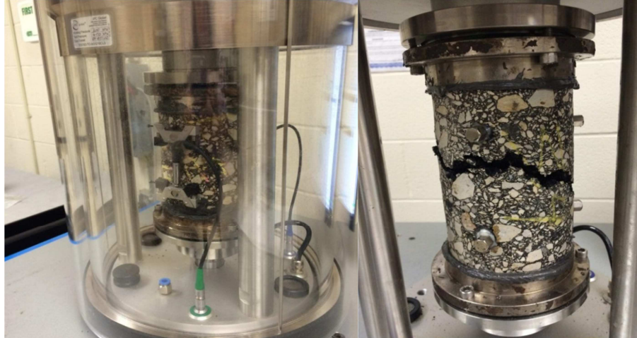
Figure 3.14 S-VECD test setup and a failed sample
