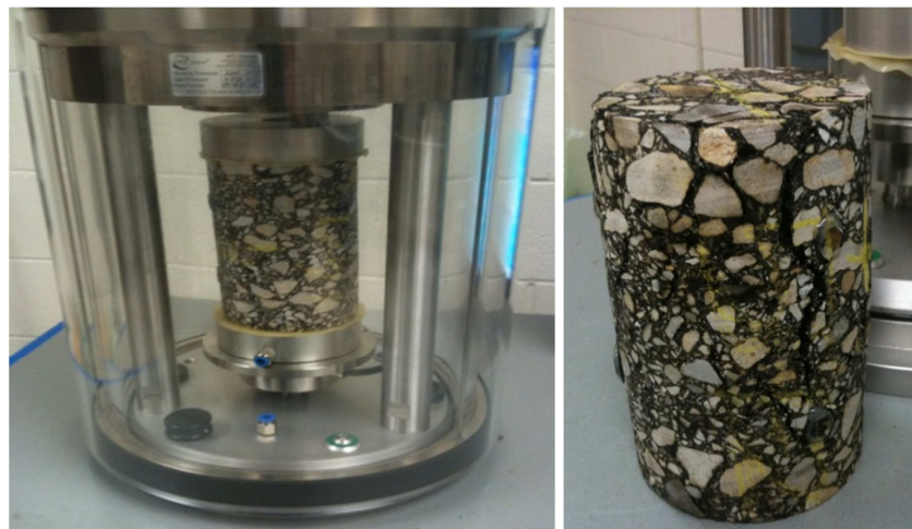
Figure 3.13 FN test setup and a failed sample
