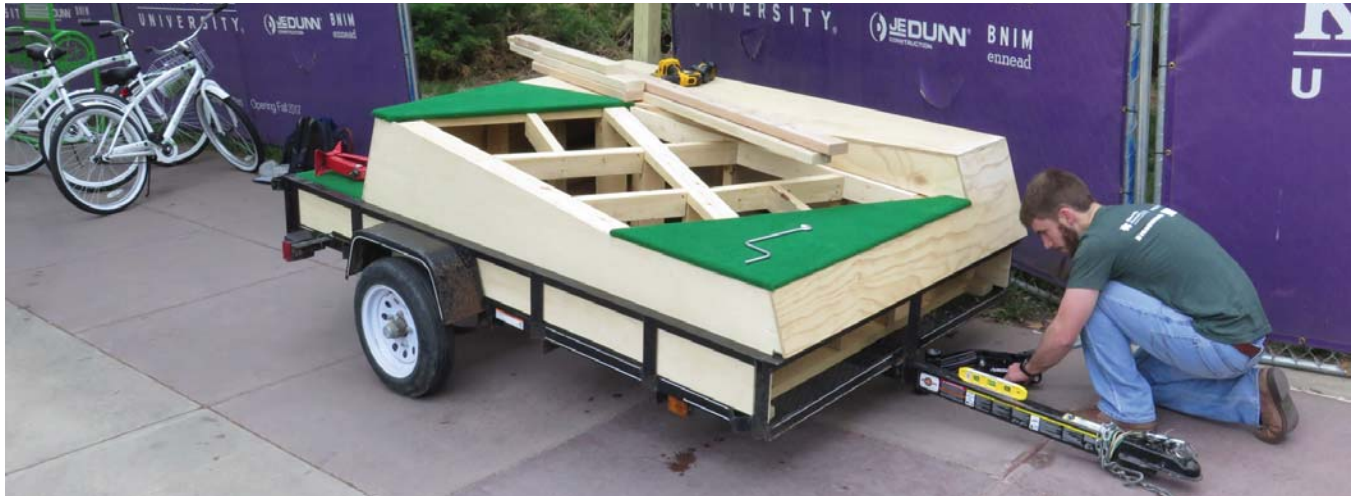
Figure 5.47: Leveling Jacks During Setup of Portable Landscape (Hahn 2016)
