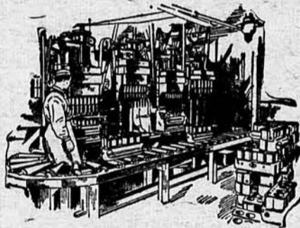
Boring and reaming valve seats in four motors at a time. The motors are locked in cast steel arms which hold them absolutely true. Consider the economy and accuracy of such manufacture.
