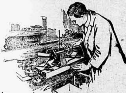
Inspecting a finished gear wheel by testing the shape of the gear to the thousandth part of an inch.
