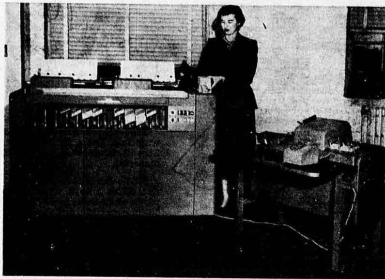
QUICK AS A WINK: Operator places census cards in Electronic Statistical Machine; note cards in sorting racks in front. This machine can sort cards into desired groups at rate of 450 a minute. Two separate printing mechanisms, similar to a typewriter carriage, allow the machine to print on a single line totals for each of 60 groups into which it can classify cards. At the same time, all information can be relayed automatically to the "Summary Punch," right, connected by cable, and punched into cards used later in still other reports.
