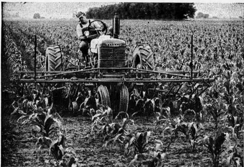
For Farmall M there's a McCormick four-row cultivator that will let you work 60 acres a day. Uneven ground is no problem: each gang floats freely up and down, and self-cleaning gauge wheels keep the gangs from working too deep. Hydraulic Farmall Lift-All gives automatic delayed action of rear sections, so that they enter and leave the ground where front sections do.
