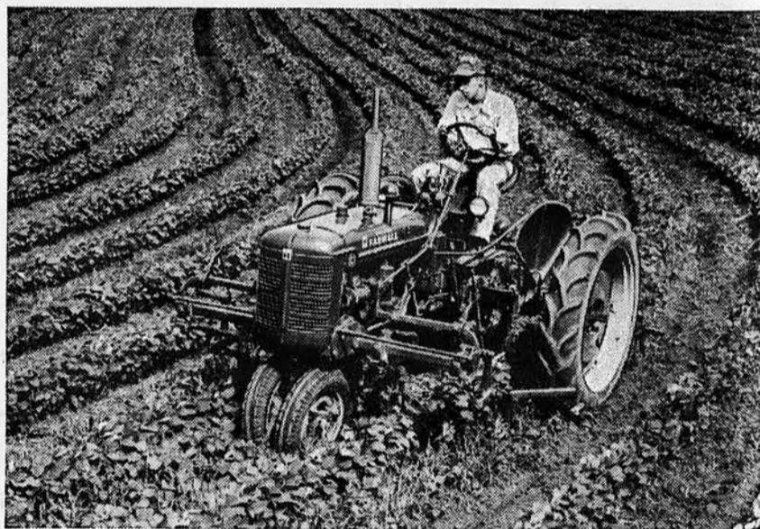
For Farmalls C (pictured), H, and M there are two-row cultivators with all the McCormick advantages. Cross-cultivating check-row corn is easy because you can see the gangs at work ahead of you... slip around an occasional out-of-line plant by giving the Farmall steering wheel a slight turn. You'll breeze through 30 acres a day with a Farmall-mounted two-row cultivator.
