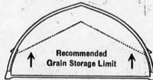
Grain storage capacity, 480 bushels per lineal foot of length in a fifty foot span.
