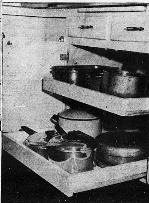
Below: Sliding shelves make larger pots and pans easy to get and double space. The kitchen floor is rubber tile—easy to clean and easy on the feet.
