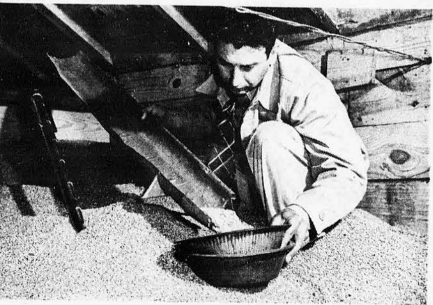
Samples of grain are dumped into a metal trough, then into a pan with a wire-mesh bottom thru which Mr. White will sift out any insects, dead or alive, and record number.
