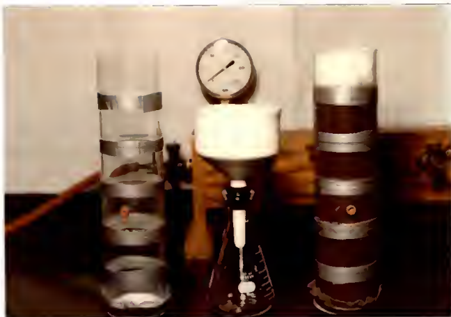
Figure 8. From left to right: soil chamber with inserted serum stopper, Buchner funnel in a 250 ml graduated filter flask, and soil column.
