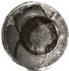
Figure 8. Top of Piston after 200 Hours of Engine Operation, Swine Digester Gas
