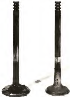
Figure 9. Face of Head after 200 Hours of Engine Operation, Swine Digester Gas
