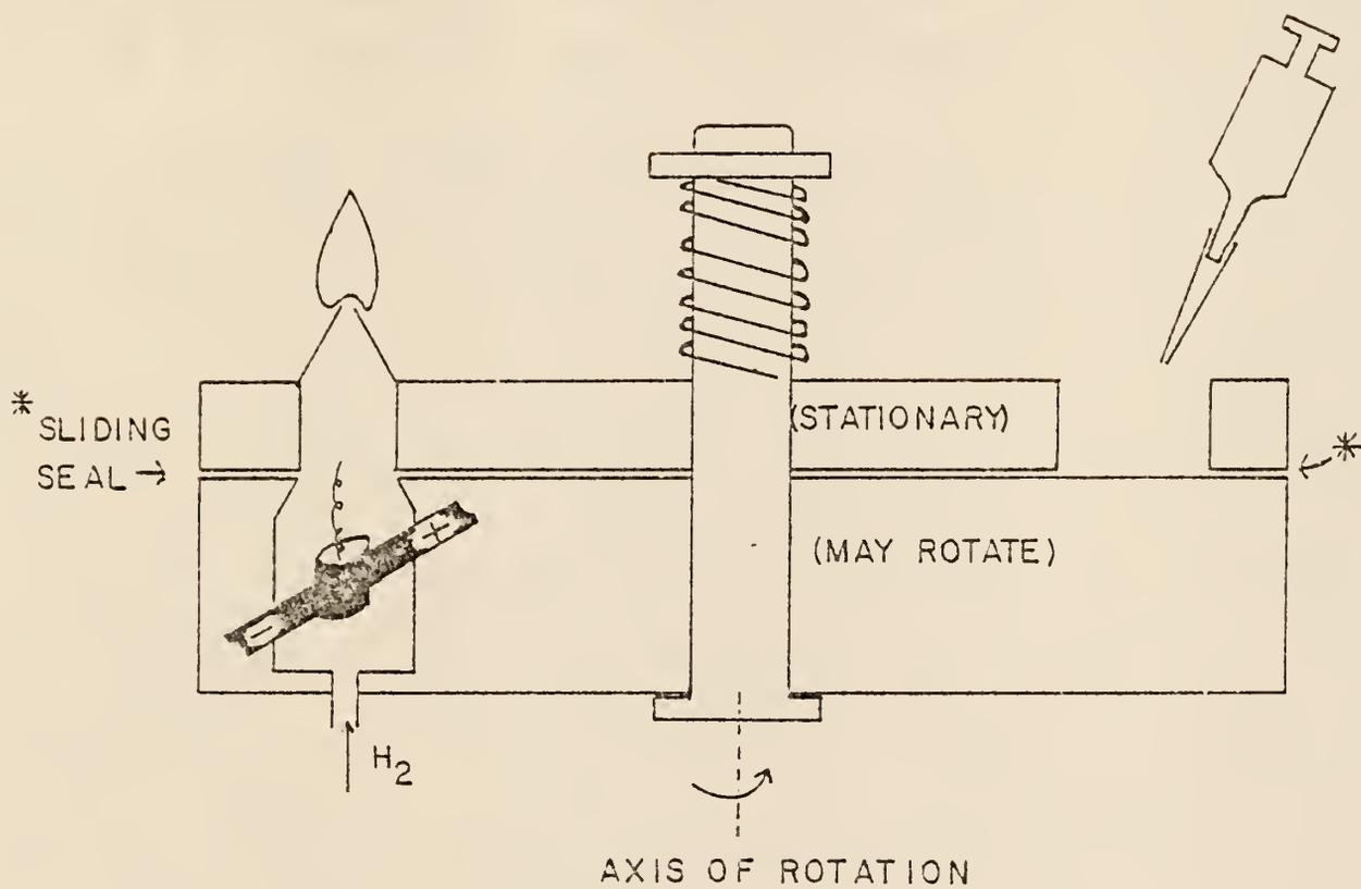
Figure 14. Miniature Diffusion Flame and Graphite Cup Atomizer;
