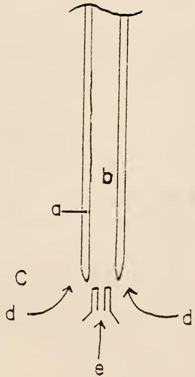
flow rates (8-12 L/min) in a nitrous oxide-hydrogen diffusion flame were unsuccessful. The flame burns only around the perimeter and not in the middle (see figure 2C).
