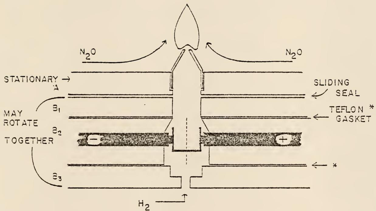
through  $B_3$  around the cup and sweeps the atom cloud into the nitrous oxide-hydrogen flame above section A. Nitrous oxide surrounds the external portions of the burner head above section A to form a laminar flame as it diffuses into the hydrogen stream emerging from the burner head.
