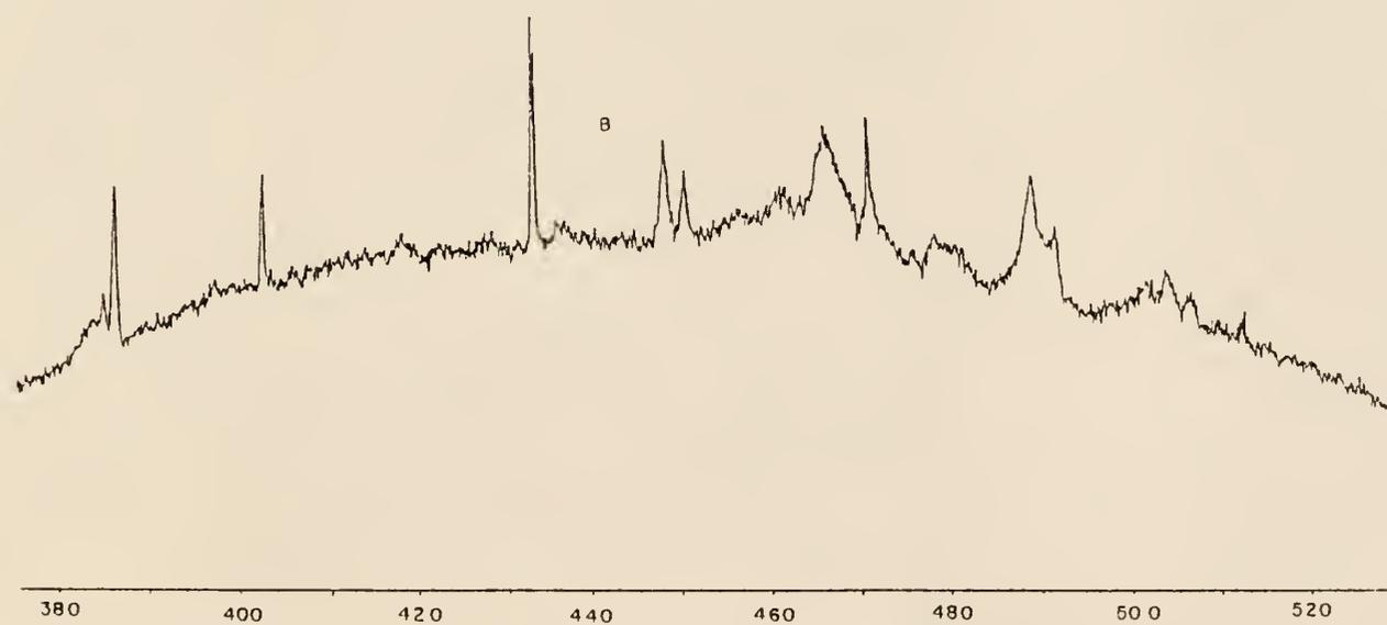
Figure 10. Fluorescence Background  $N_2O/H_2$  premixed flame
