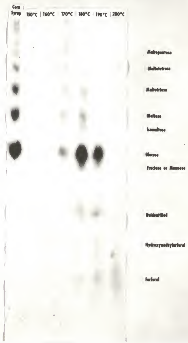
Fig. 2. Chromatogram showing effect of temperature of heat treatment (°C) on sugar production.
