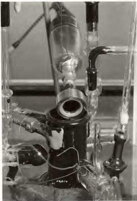
Fig. 6 Surface - barrier radiation detector before insertion into operating position .
