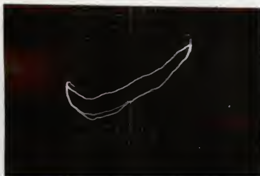
Fig. 7. Oscilloscope patterns for the three specimens, showing the change in the voltage drop across the whisker as a function of the applied voltage.
