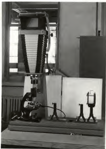
Fig. 3. The microscope and camera used in this study. (A) Bausch and Lomb photomicrographic camera model L with Poloroid Land Back camera attachment. (B) Bausch and Lomb student series microscope. (C) Heating stage for accurate temperature control.
