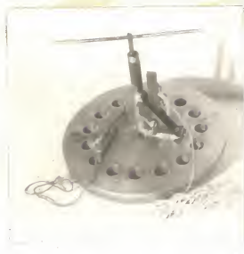
Fig. 7. The cover plate with the firing device. The hammer is in cocked position, and the safety plate has been swung out of "safety" position. The hammer is released by pulling the trip to the right.
