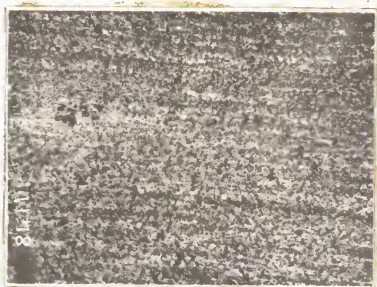
Fig. 22. Photomicrograph of a cold rolled specimen deformed 78.5% (trial No. 10, Table 9). The extreme fragmentation of the grains and consequent grain refinement is noticeable. Etched, 500 X.
