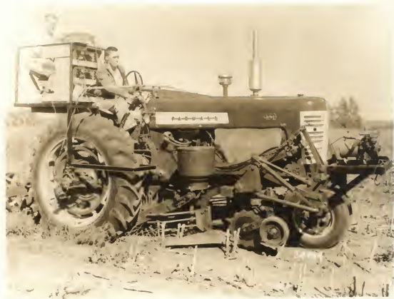
Fig. 6. The tractor as it was equipped for till-planter power requirement testing.
