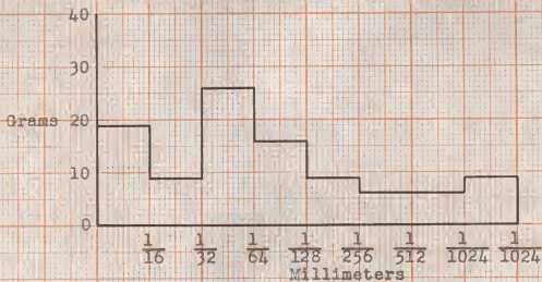
Fig. 70. Histogram showing the distribution of particle size of sample no. 3P.
