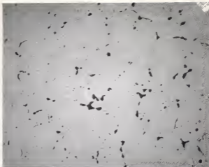
Fig. 32. Magnesium, zinc, and calcium alloy. 4 per cent Zn., 0.1 per cent Ca. X 100. Heat treated at 770° F.
