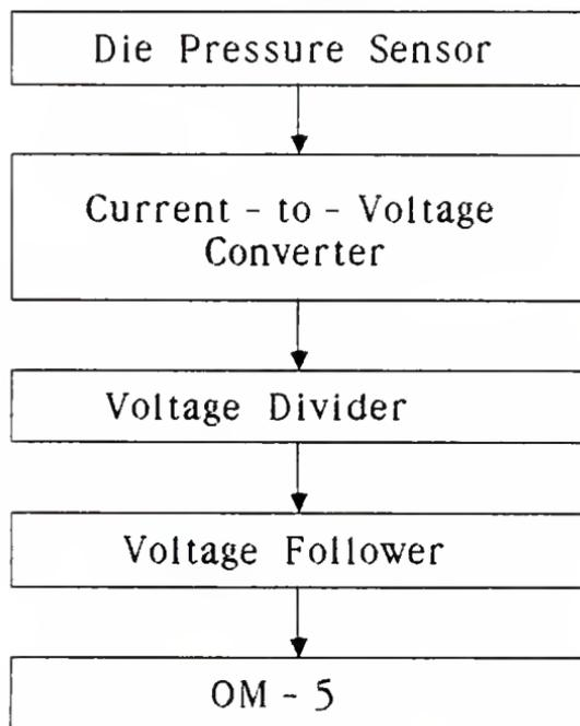
Figure 3.11 Block Diagram of Die Pressure Sensor Interface
