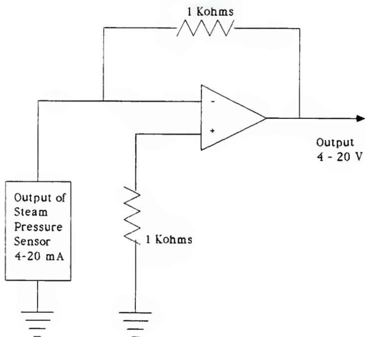
Figure 3.7 Schematic Circuitry of Current-to-Voltage Converter
