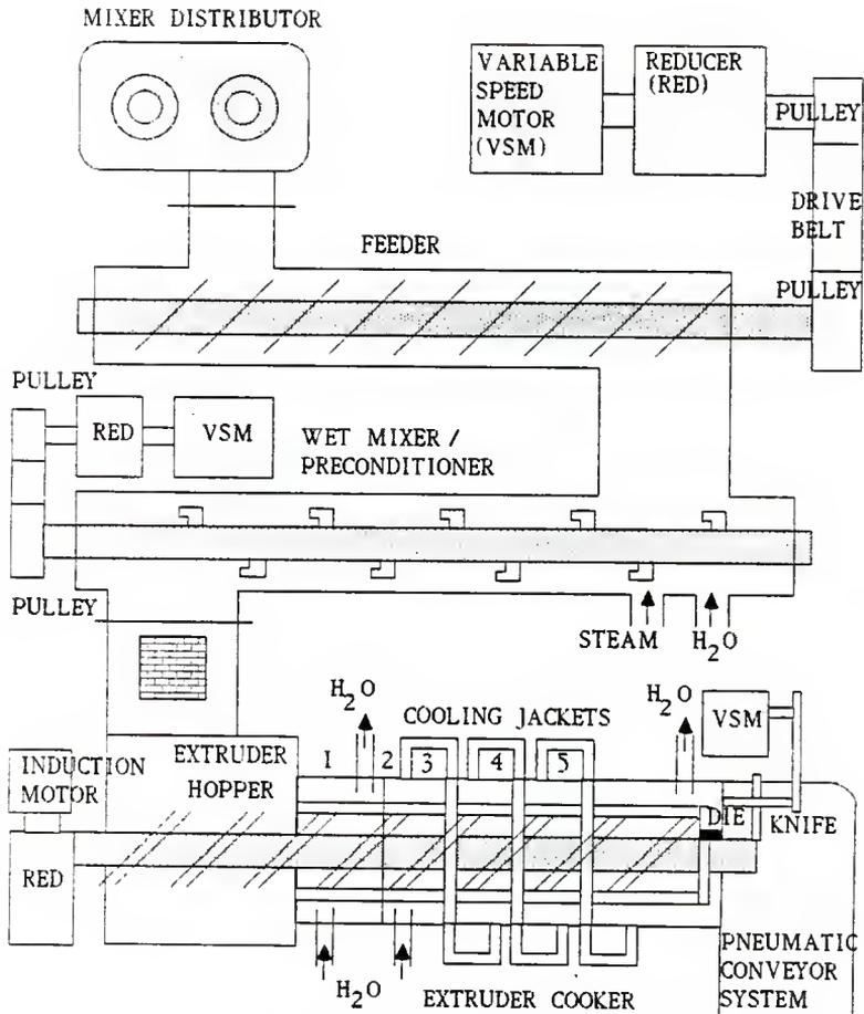
Figure 2.1 General Diagram of an Extrusion Cooking process System
