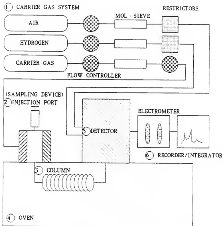
Figure 2.7 Block Diagram of a Gas Chromatography System
