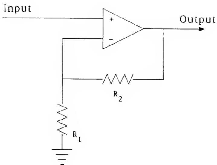
Figure 3.9 Schematic Diagram of Non-inverting Amplifier
