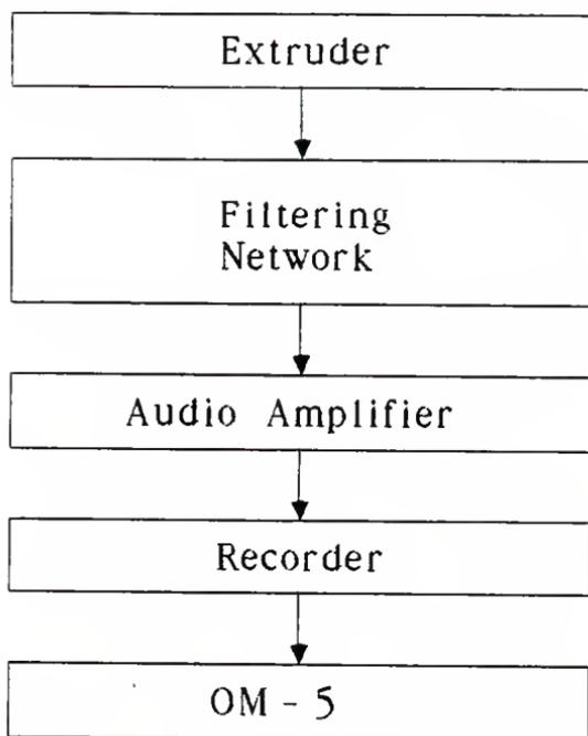
Figure 3.12 Block Diagram of Audio Sensor Interface
