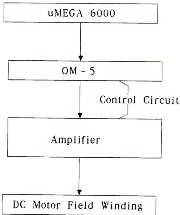
Figure 4.3 Block Diagram of the Control Circuit and the DC Motor Field Winding
