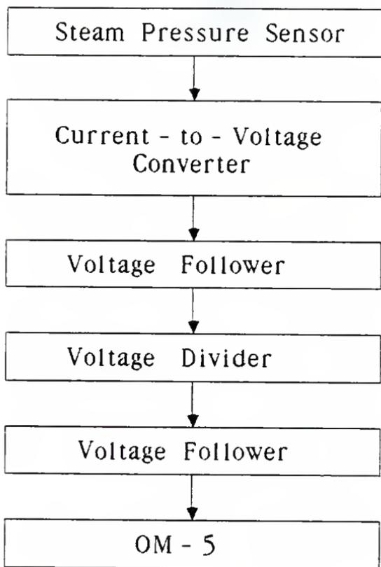
Figure 3.6 Block Diagram of Steam Pressure Sensor Interface
