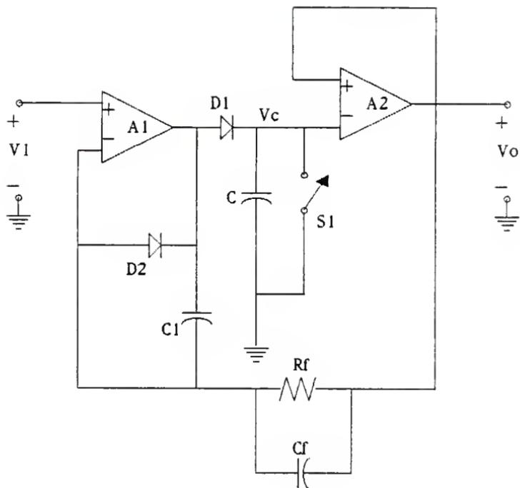
Figure 3.5 Schematic Circuitry of Peak Detector
