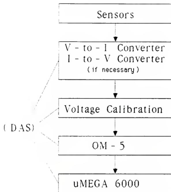
Figure 2.6 Block Diagram of Sensors Interfacing with DAS
