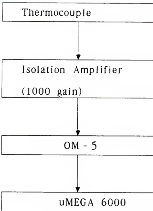
Figure 3.8 Block Diagram of Thermocouple Interface
