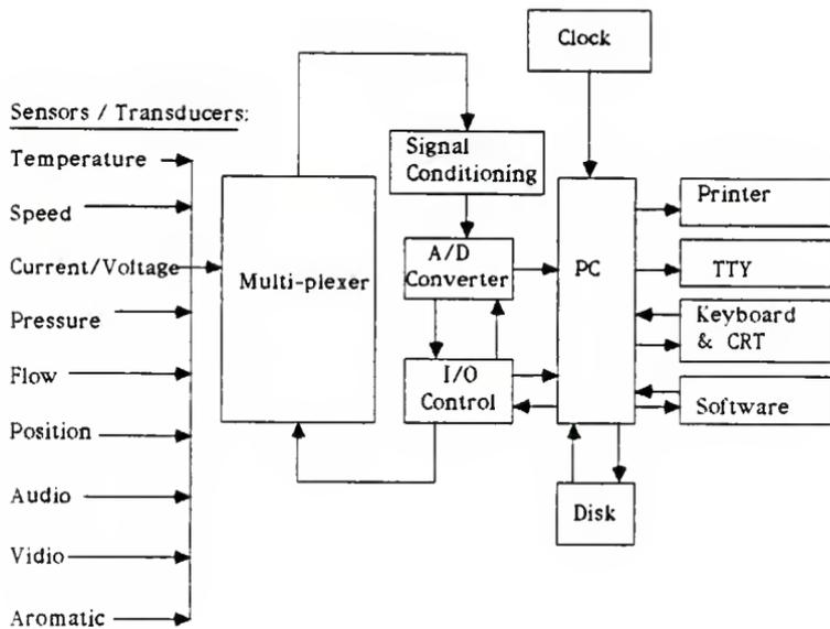
Figure 2.4 Interface Configuration Between Sensors and PC
