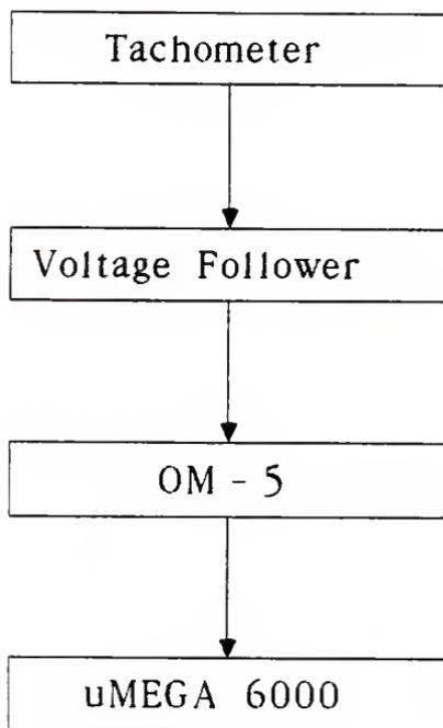
Figure 3.3 Block Diagram of Tachometer Interface
