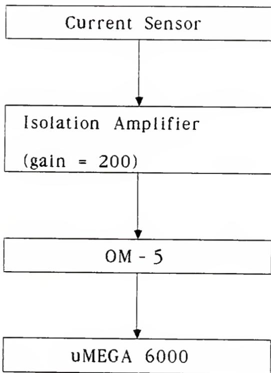
Figure 3.10 Block Diagram of Current Sensor Interface
