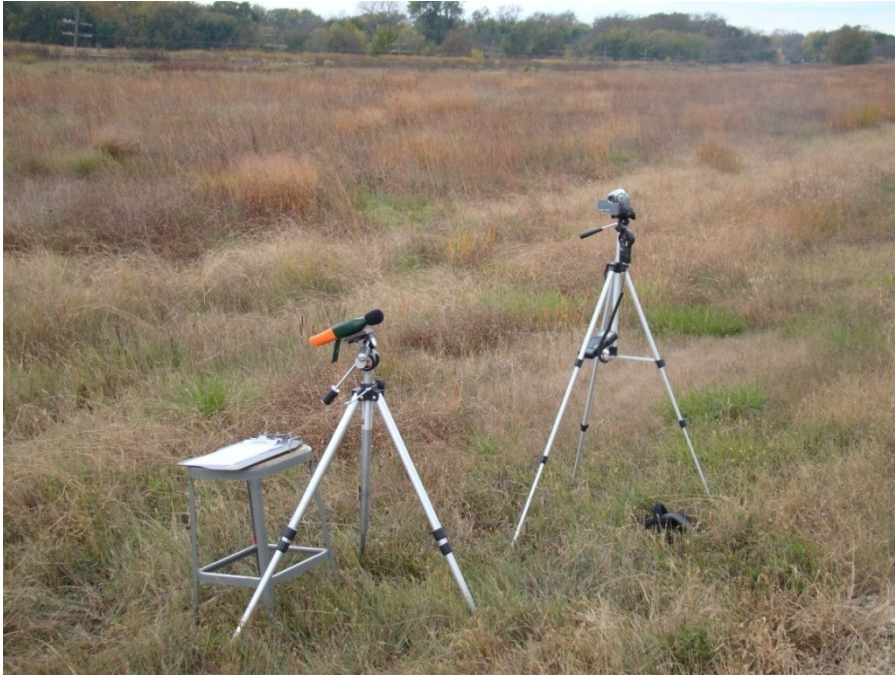
Figure A1: Experimental setup; Ex-Tech sound level meter and Sony camcorder
