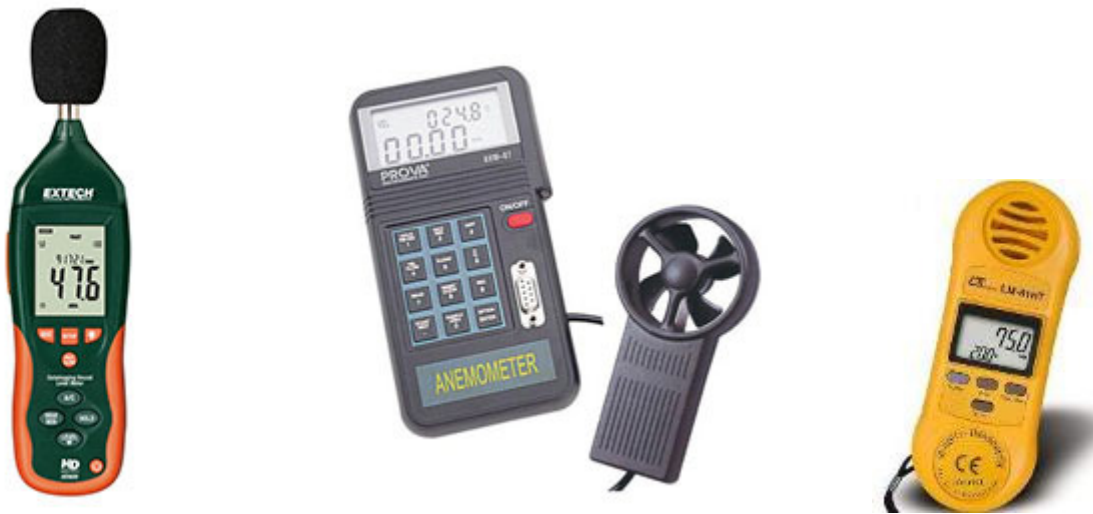
Figure 3.3 Ex-Tech HD 600 sound level meter, PROVA Anemometer and CE LM-81HT thermometer / anemometer / humidity meter
