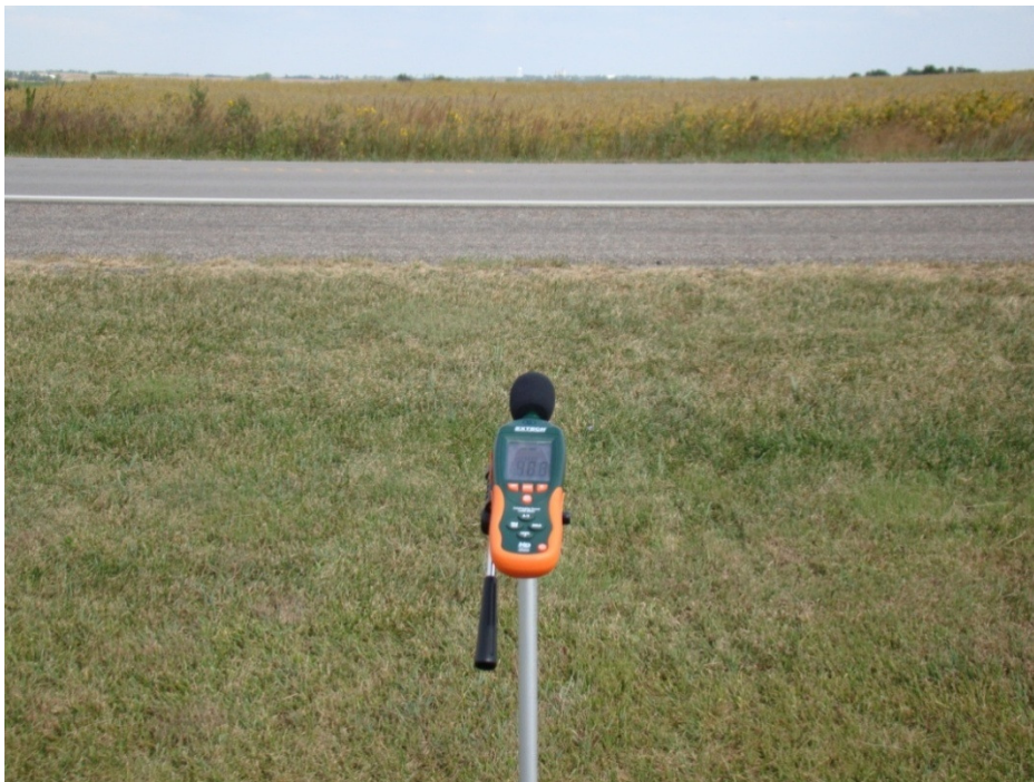
Figure A2: Position of sound level meter with respect to the highway.
