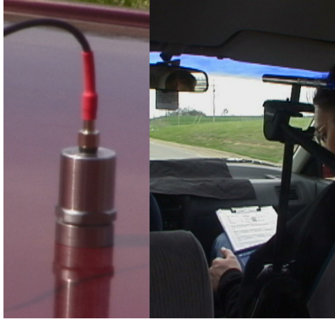
Figure 2.5: Accelerometer (Left) and Microphone (Right) (Meyer and Walton, 2002).
